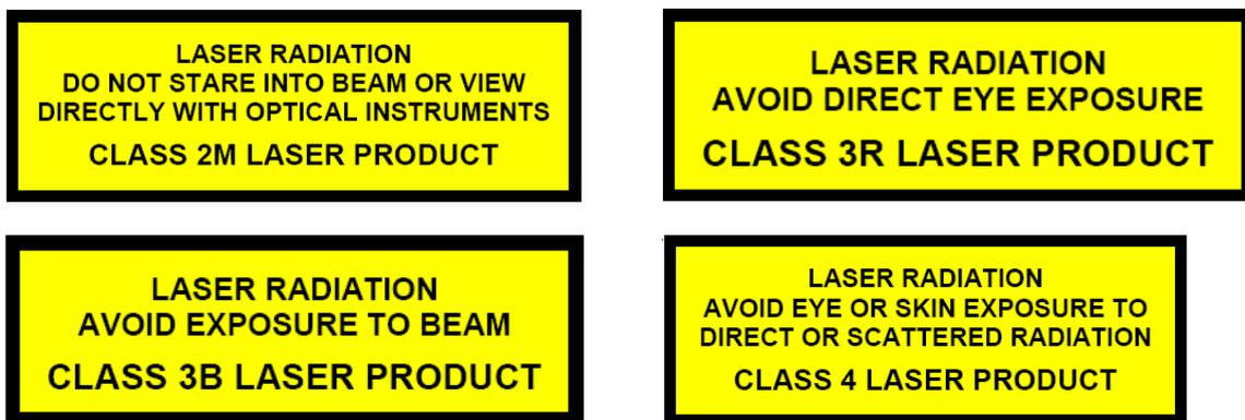
**Figure 9-6: Labelling used on laser systems to indicate class and risk.**
