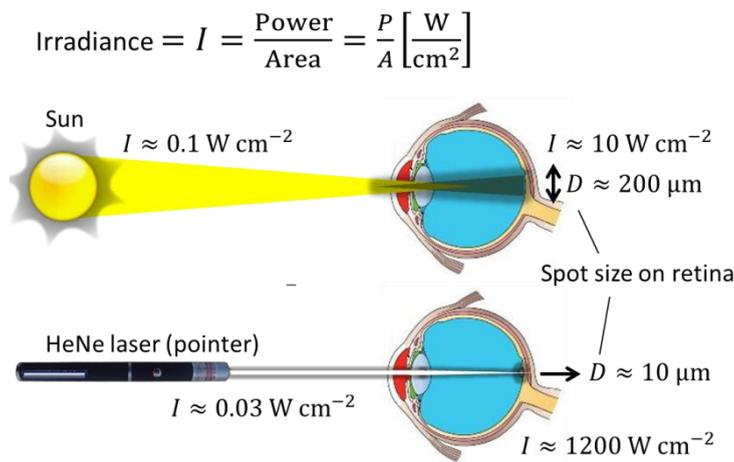
**Figure 3-1: Comparison of the irradiance of the sun and a 1mW laser (2 mm beam diameter) on the retina.**
