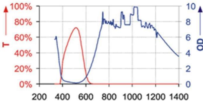
**Figure 9-9 Transmission and optical density of a filter used in a set of laser eye protection.**
