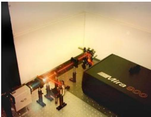
**Figure 6-8 Pulsed Ti:sapphire laser system.**
