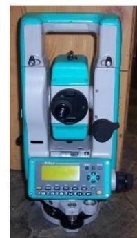
**Figure 6-5: Modern theodolite with Class 2M built in.**
