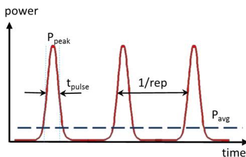
**Figure 7-1: Illustration of a laser pulse.**
