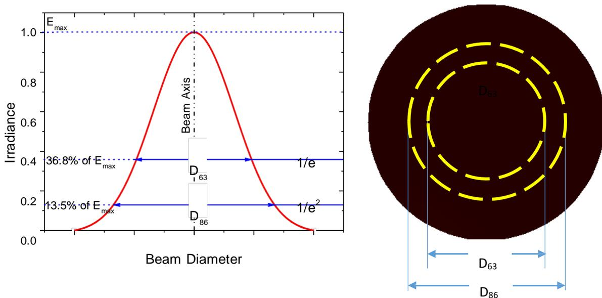
**Figure 7-3: Normalised intensity profile of a Gaussian laser beam showing the cut off points used to define the beam diameter. On the right hand side an illustration of the transverse beam profile is shown where approximate positions of the  $D_{63}$  and  $D_{86}$  diameters are indicated.**
