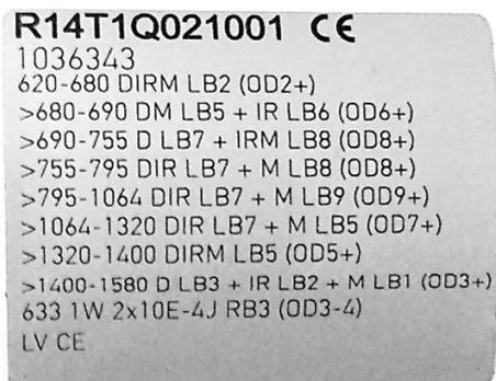
**Figure 9-8: Example of a label on laser safety goggles.**
