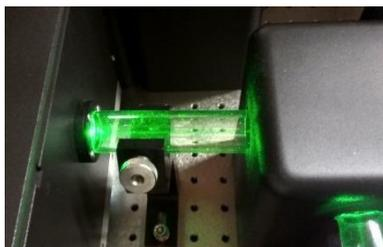
**Figure 9-3: High powered laser with an enclosed beam path.**
