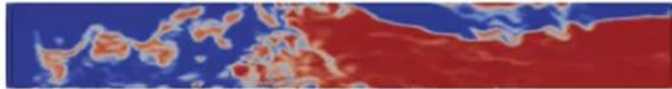
Sample output from the CFD simulation showing water (in red) and air (in blue).
