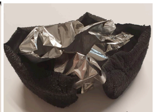
Fig. 3: ASR & aluminium laminated pouches (middle) and Tetra Pak (right) post RecEOL recycling.
