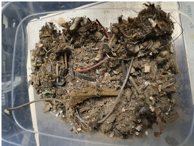
Figure 4 - Automobile shredder residue before treatment by the RecEOL reactor. The RecEOL technology removes any plastics and other volatile materials such as residual oil turning the material from a hazardous waste to a benign waste.
