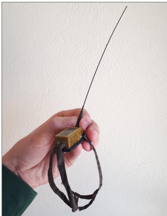
Plate 1. Platform Transmitter Terminal (satellite transmitter) and harness (neck loop and chest strap) used in the current study.
