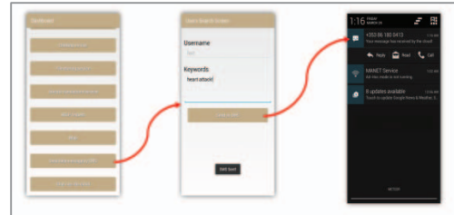
Figure 8. Sending a HELP request via SMS (user's side) using the Android app
