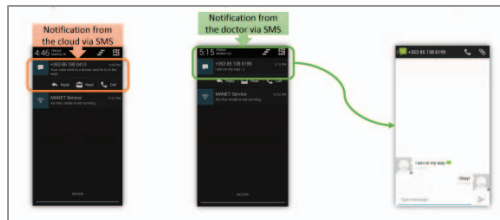
Figure 10. SMS notification is sent from the cloud to the requester side using the Android app
