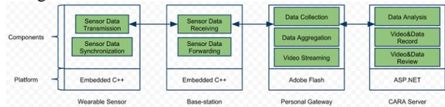
Figure 2. Software Architecture
