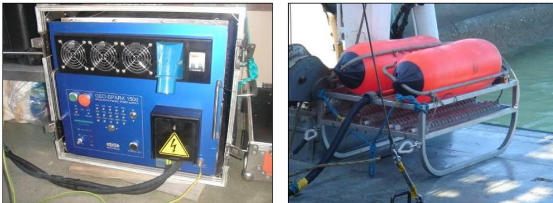
**Figure 7. Sparker Seismic System**
