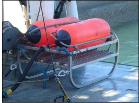
Hull mounted ESE 5001S 3.5 kHz pinger system
