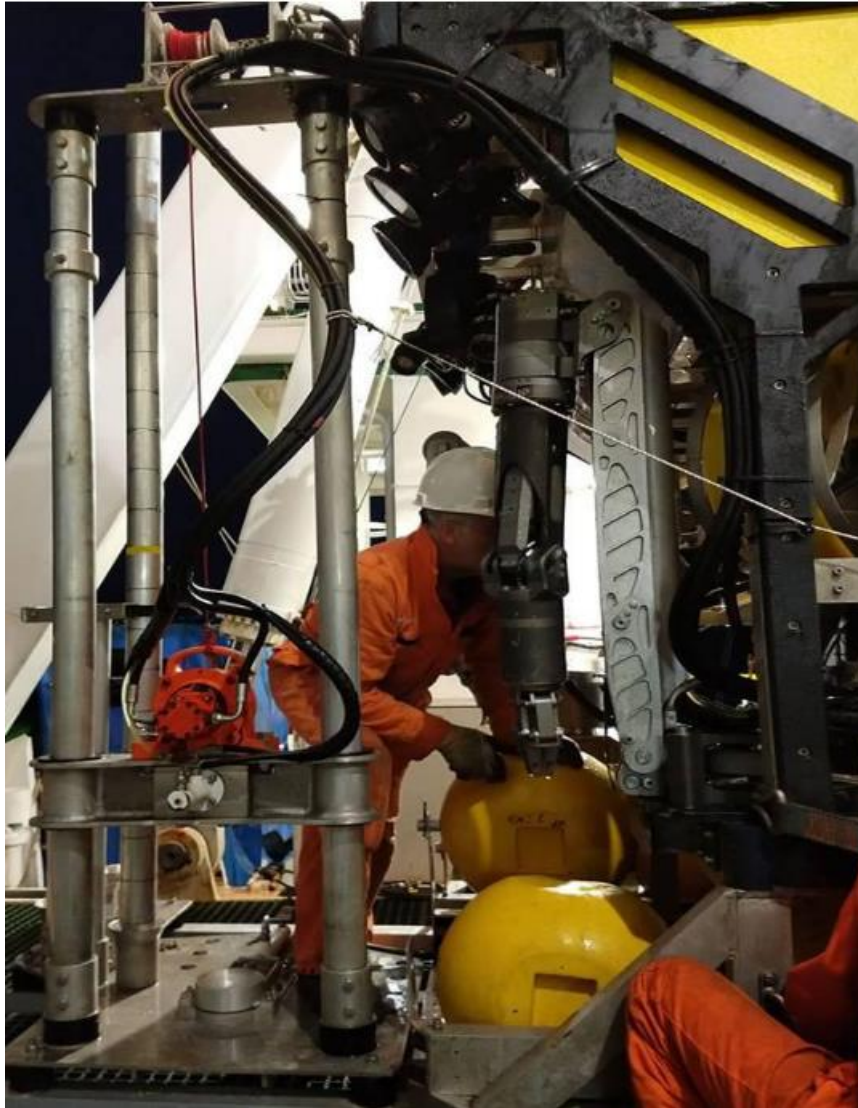
The Vibrocore rig mounted on the ROV
