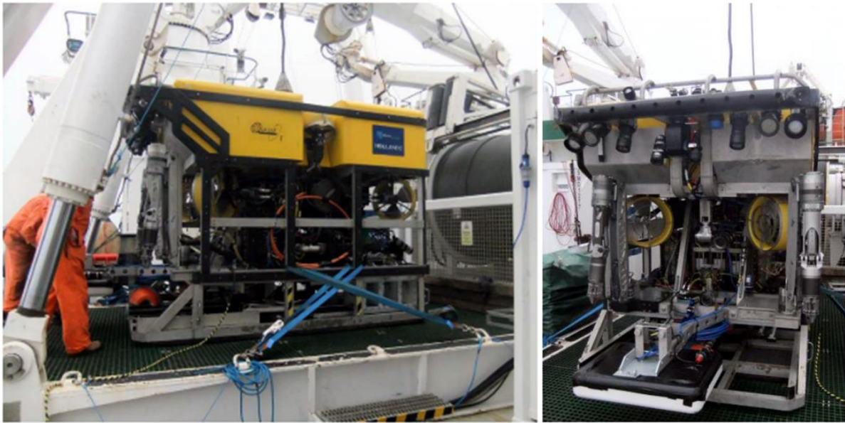
The Holland 1 ROV being prepared for launch (left) and its video and lighting rig (right).
