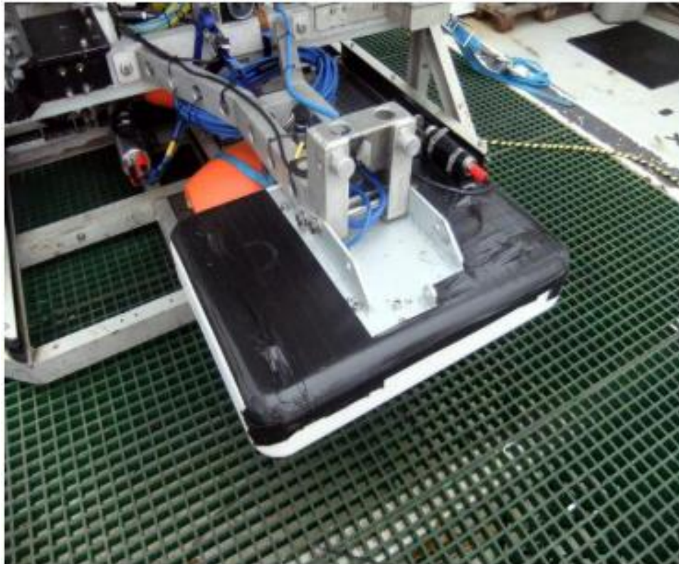
Kongsberg EM2040 mounted on the Holland 1 ROV
