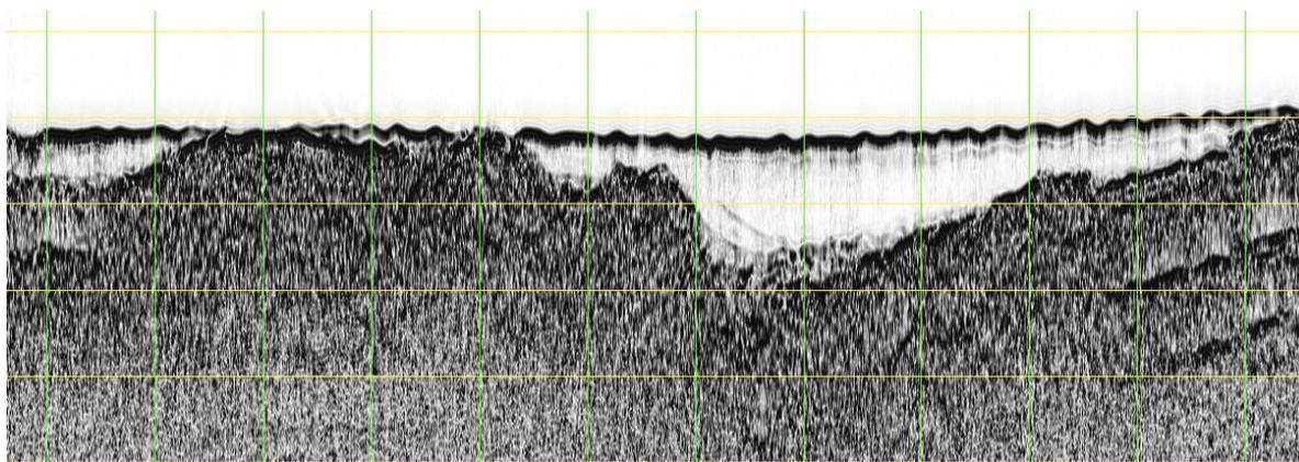
Figure 11. Sub-bottom profiler line from the South Sound (Line 2) showing dipping bedrock (probably limestone) with hollows partially filled by the lower unit (fluvio-glacial) overlain by upper unit. Vertical scale is 10m
