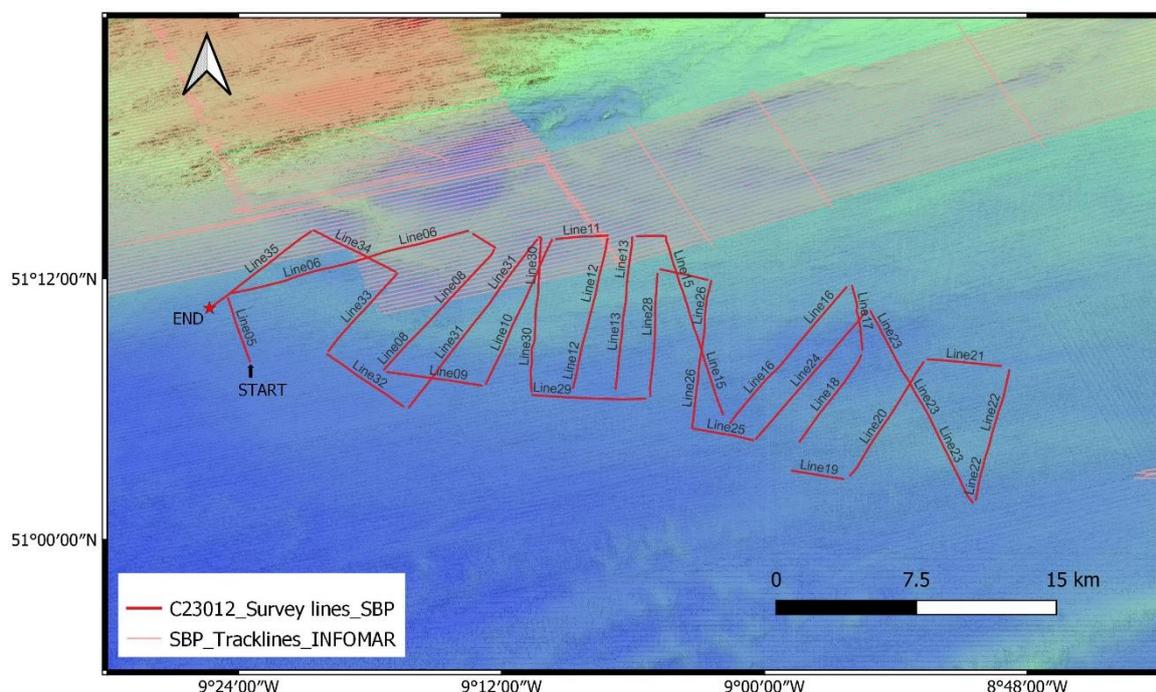
Figure 18: The sub-bottom profiler survey lines in Celtic Sea.
