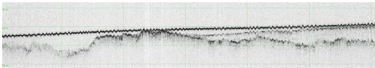
Figure 15. Sub-bottom profiler line from the North Sound (Line 43) showing bedrock overlain by the lower unit (right-side) and the upper unit overlying all.
