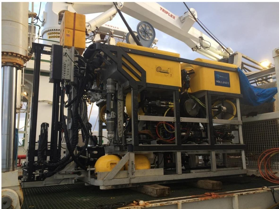
*Figure 4. Holland 1 Remotely Operated Vehicle with the Williamson ROV rockdrill attached at the front*
