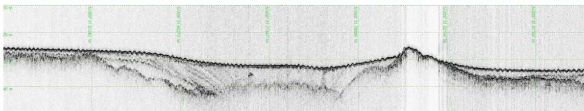
Figure 14. Sub-bottom profiler line from the North Sound (Line 47) showing more rounded bedrock (probably granite) overlain by a migrated channel fill and thick upper unit
