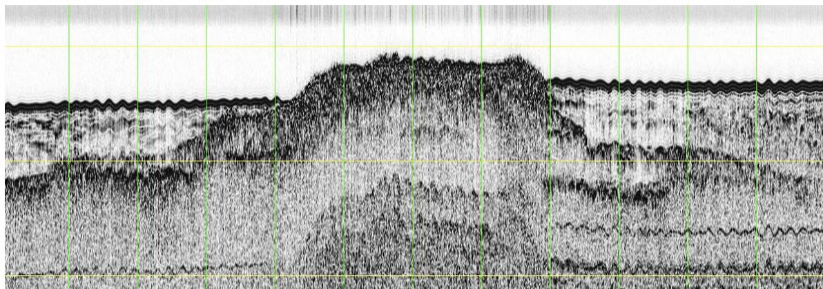
Figure 12. Sub-bottom profiler line from the Inner Bay (Line 32) showing bedrock rising above the seabed surrounded by the lower unit (fluvio-glacial) with a thin veneer of upper unit (Holocene marine sediment)
