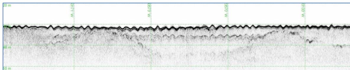
Figure 19 The sub-bottom profiler section showing a thin transparent 1<sup>st</sup> acoustic reflector and an U-shaped 2<sup>nd</sup> reflector characteristic of a recessional moraine.
