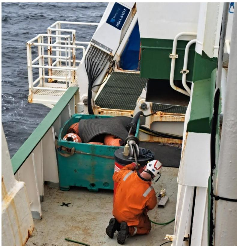
Figure 9. ROV crew re-terminating the umbilical
