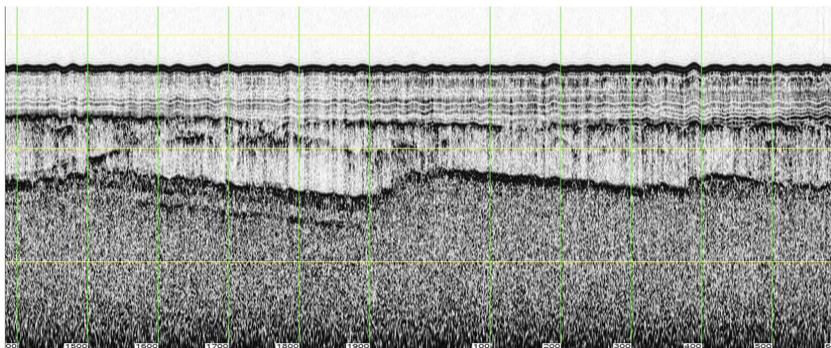
Figure 13. Sub-bottom profiler line from the Mid Bay (Line 7) showing dipping bedrock with clifflets overlain by the lower unit (fluvio-glacial) with parabolic reflectors from boulders and some internal structures. This is overlain by a thick upper unit (Holocene marine sediment) which is more stratified at the base.
