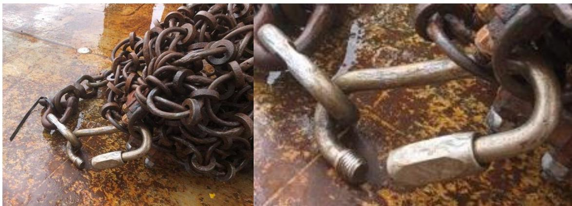
*Figure 10. Damaged shackle attaching the dredge to the cable. Closed up shows the shredded threads of the screw*
