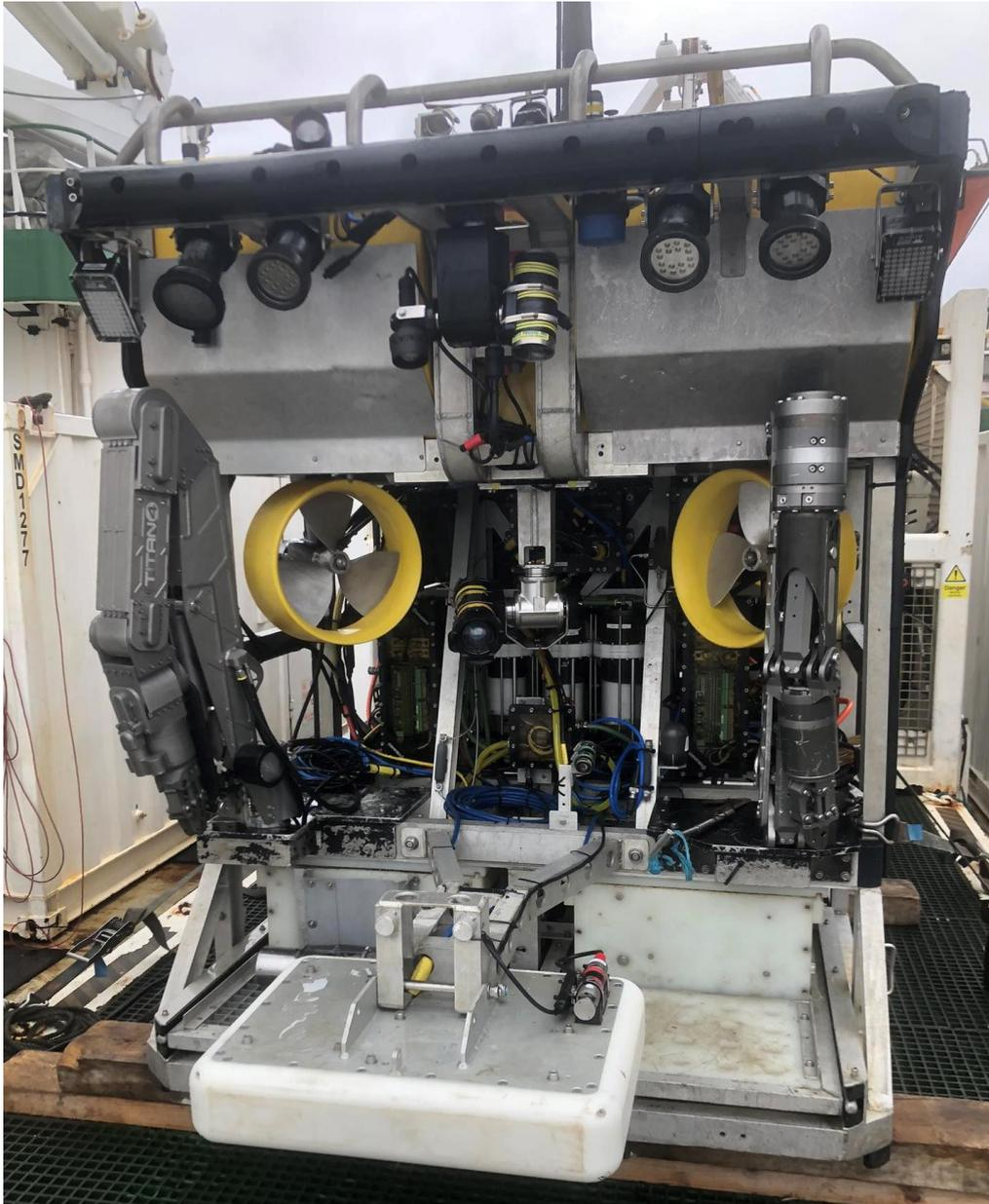
Figure 5. *Holland 1 Remotely Operated Vehicle with the EM2020 multibeam echosounder head install on the front*
