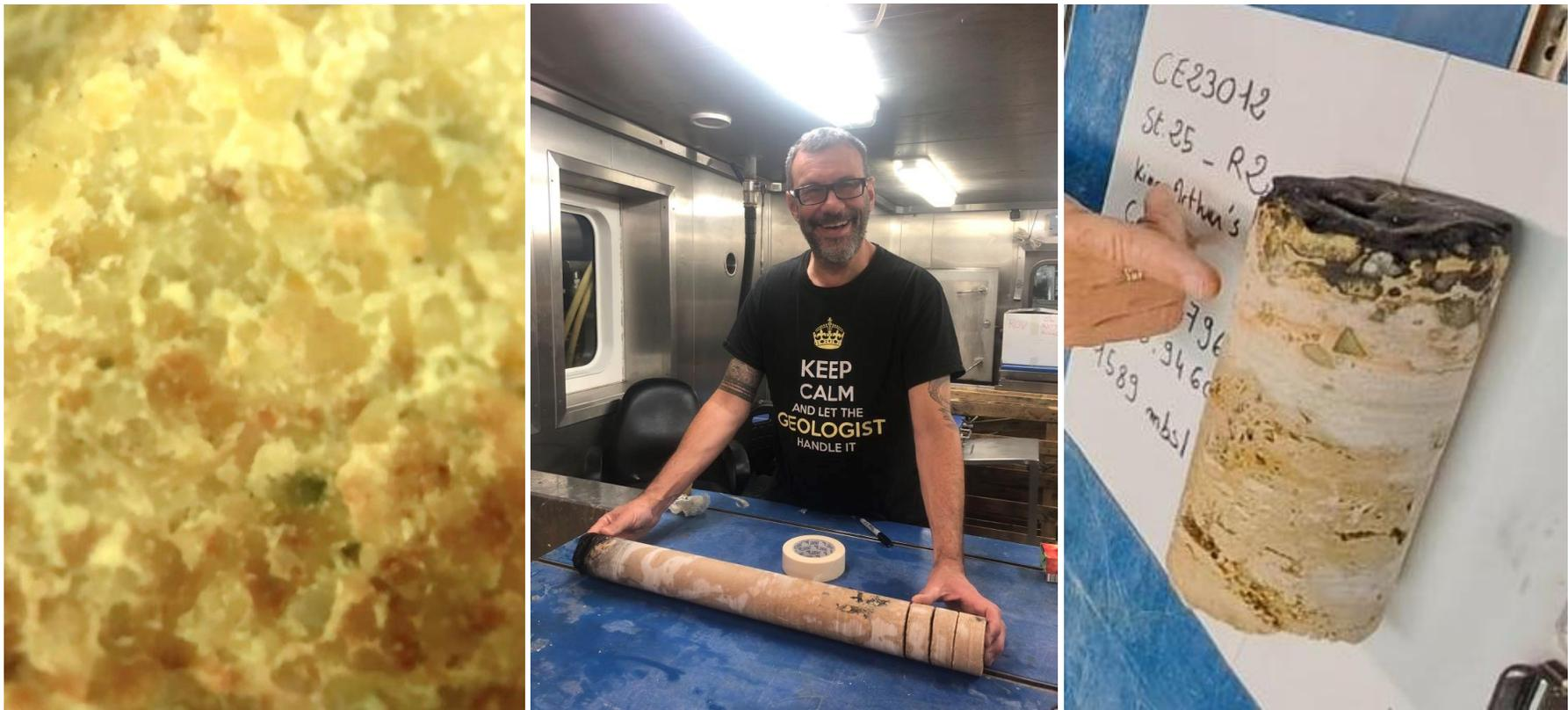
Figure 51. Left and Middle: **St19\_R1**: 71 cm long core consisting of a massive, well sorted, angular quartz arenite (sandstone). Right: **St25\_R2**: 16.5 cm long core consisting of sparite (limestone) overlain by a calcareous matrix-supported breccia and metaliferous oxide crust.
