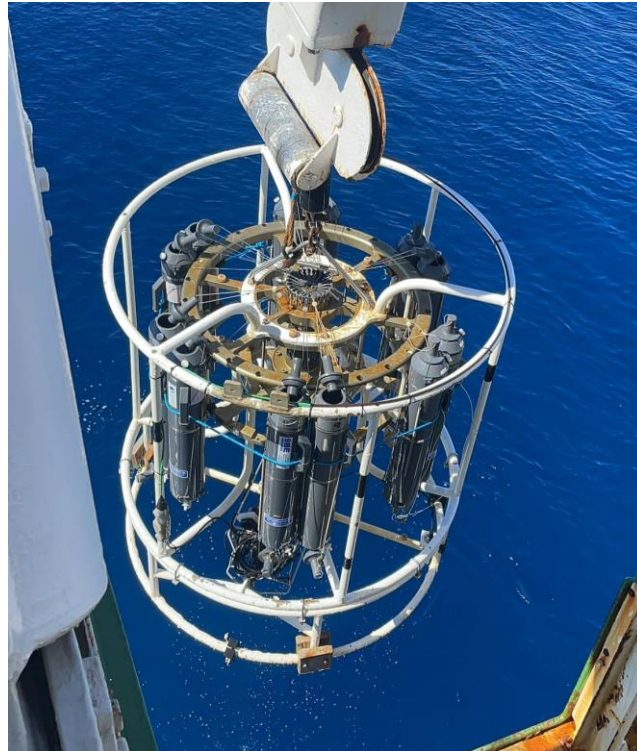
Figure 5. Sea Bird Electronics SBE 911 plus CTD
