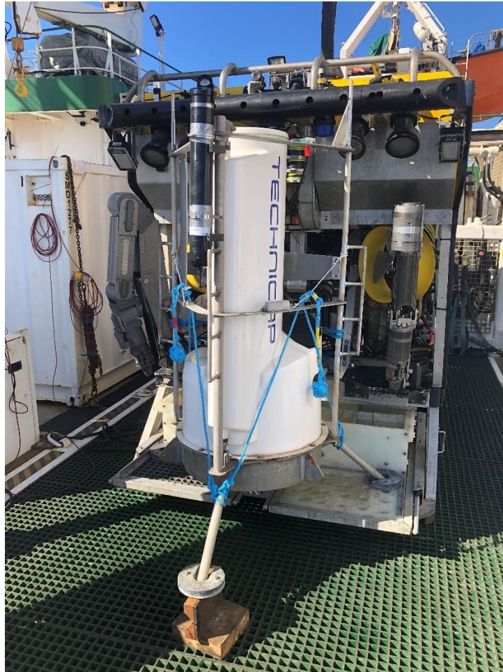
Figure 4 Little MonSta lander “Charlotte” ready for deployment on the front of the Holland 1 ROV
