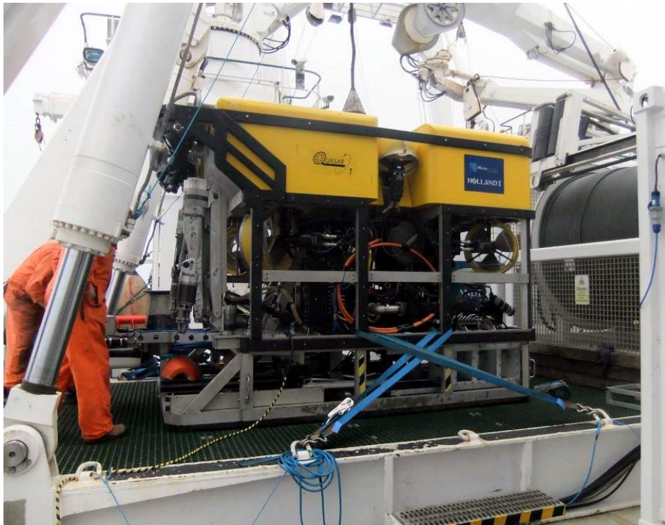
The Holland I ROV on deck (portside view), teh aspirator tank is at the lower back
