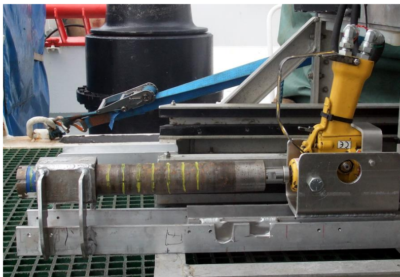
Rock drill mounted on the ROV
