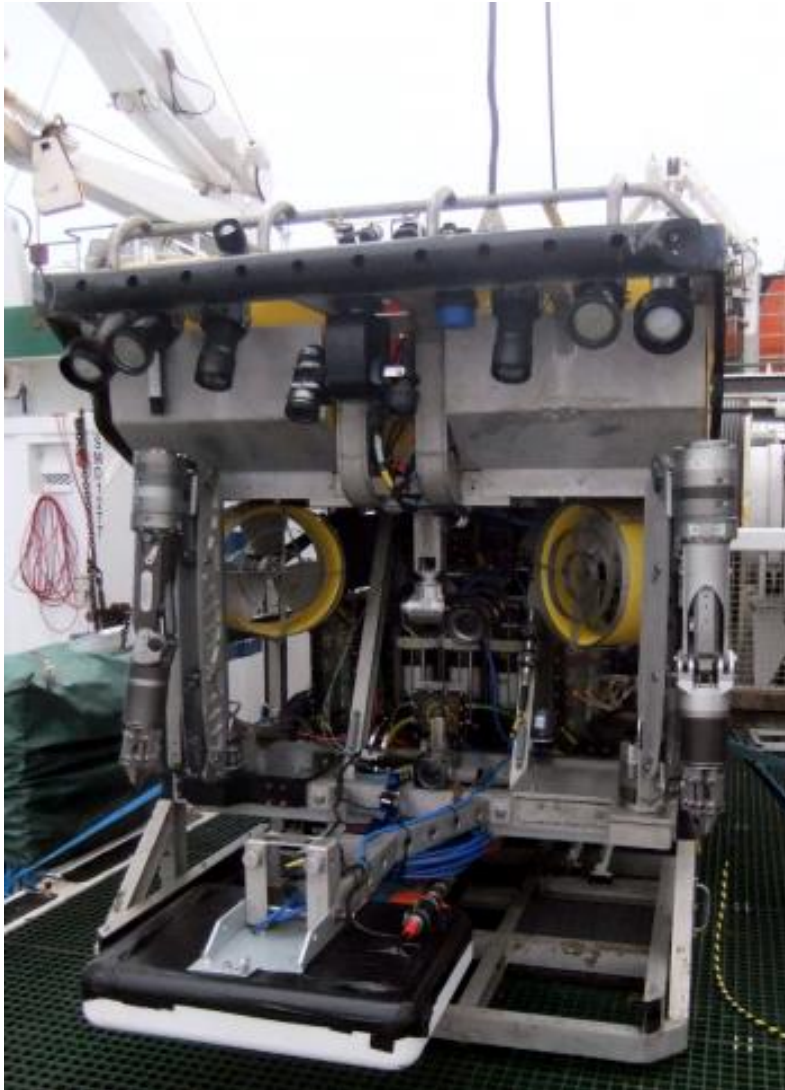
The Holland I ROV front view showing the cameras, lights, robotic arms and EM2040 MBES mounted at the front
