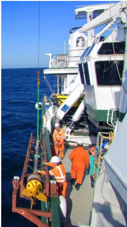
6m gravity corer
