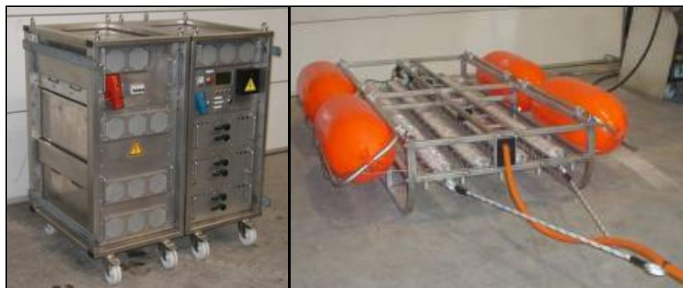
*Figure 4. Geo-Spark 6 kJ pulsed power supply and towed Geo-Source 400 Sparker source*
