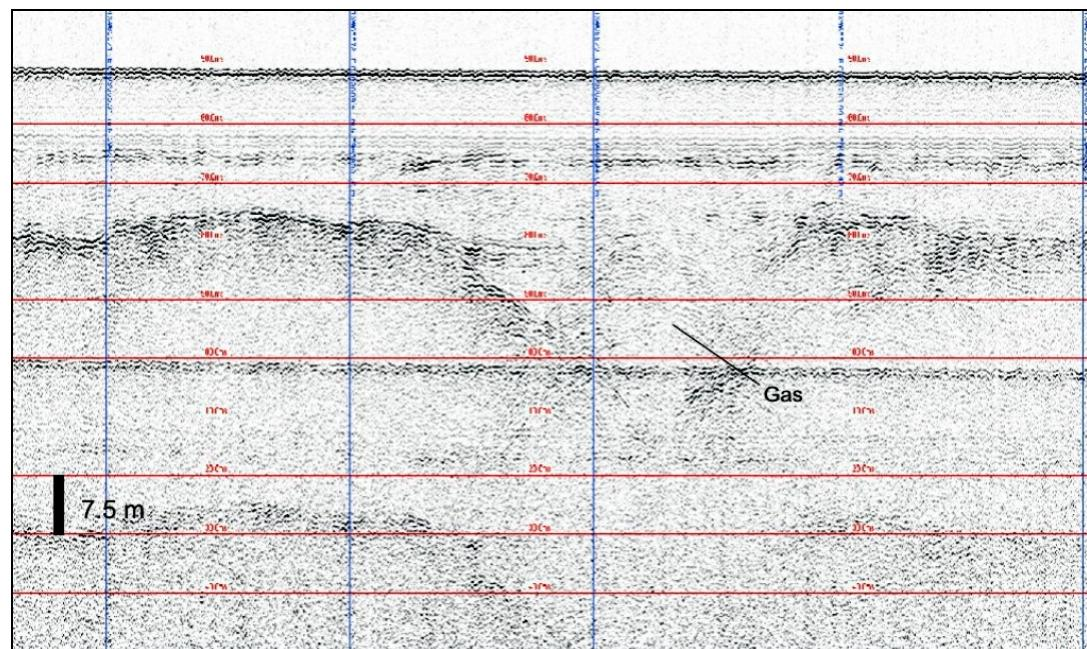
Figure 20. Seismic image from the Northern Mudbelt showing the accumulation of shallow gas.
