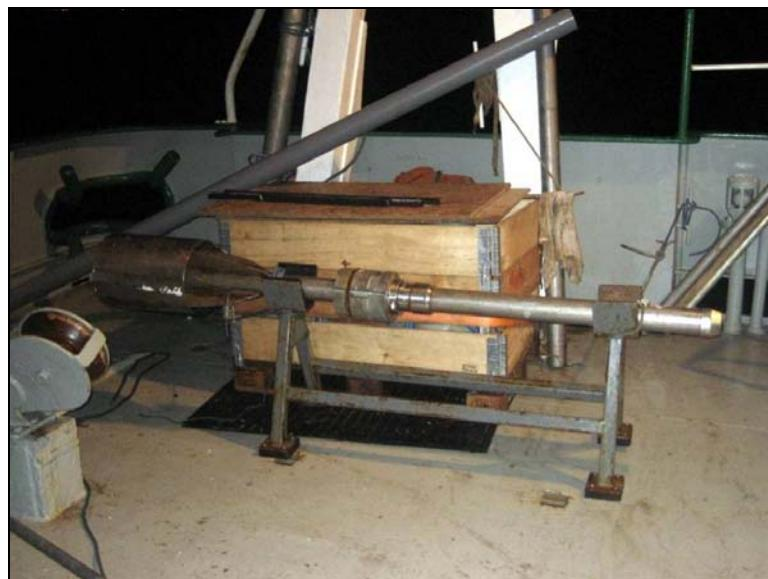
*Figure 9. Gravity corer with 1 m core barrel*
