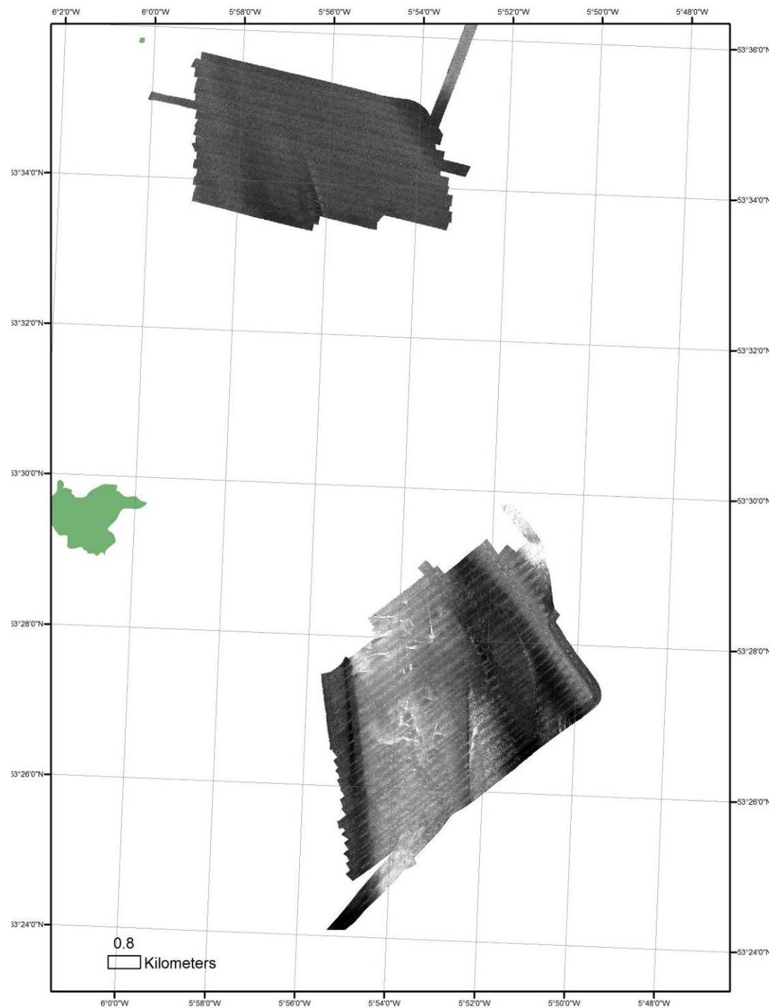
*Figure 31. Contrasting backscatter from the Rockabill (north) and Lambay (south) areas due to difference in grain-size (sandier in Lambay) and exposure of lithified sediments in Lambay.*
