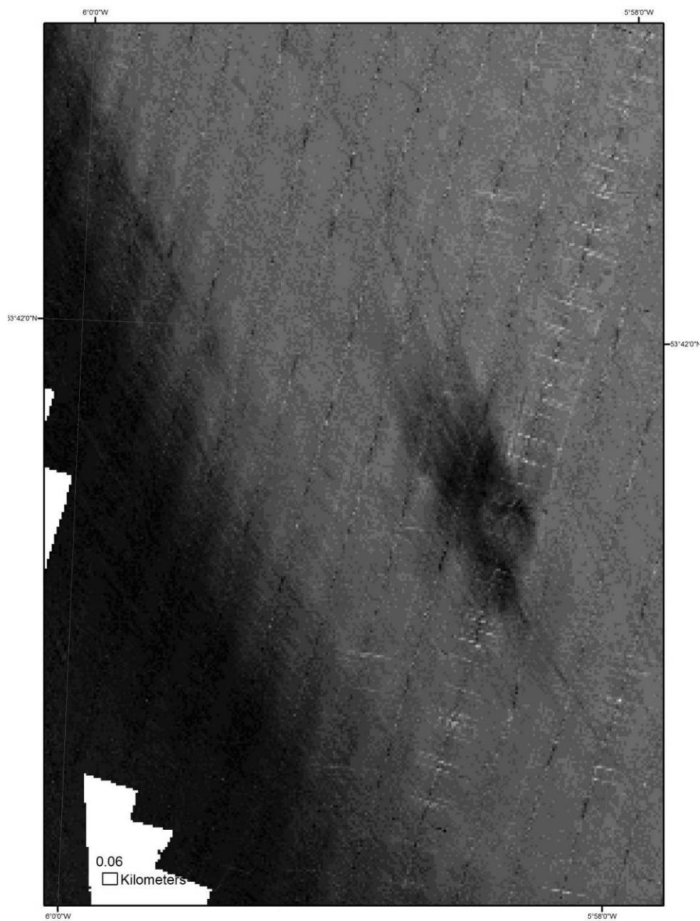
*Figure 14. Multibeam backscatter image showing another pockmark (dark irregular backscatter in the central image) and a zone of high backscatter in the south of the area. The reason for the change in backscatter may be due to an increase in silt content in the pockmark or cementation. The zone of dark backscatter to the southwest may also be due to gas although this is unclear at present.*
