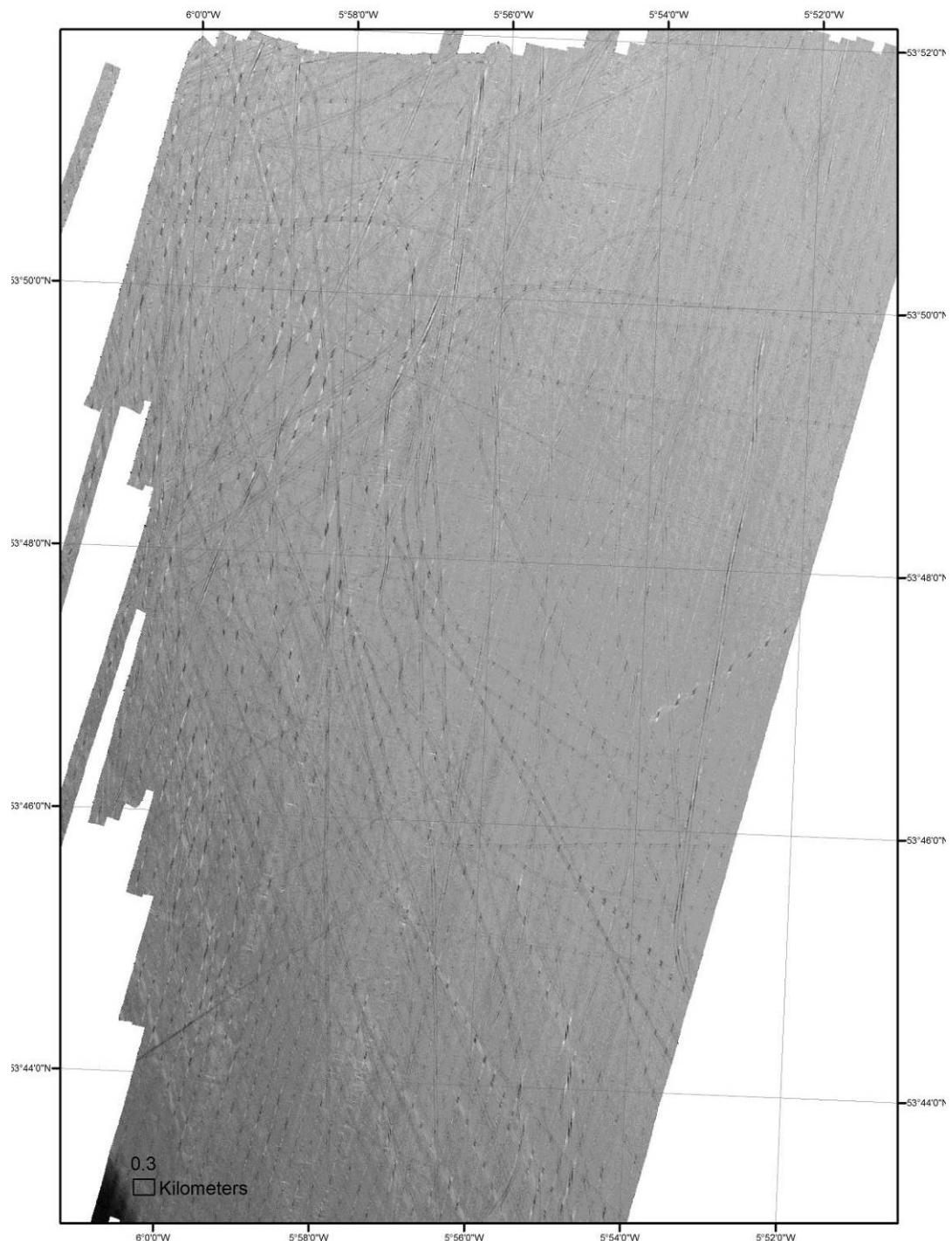
*Figure 15. Multibeam backscatter in most of the Northern Mudbelt showing trawl-marks caused by prawn fishing. Areas of more intense trawling are apparent. It is not known how long a trawl marks remains visible on the seabed in this area.*
