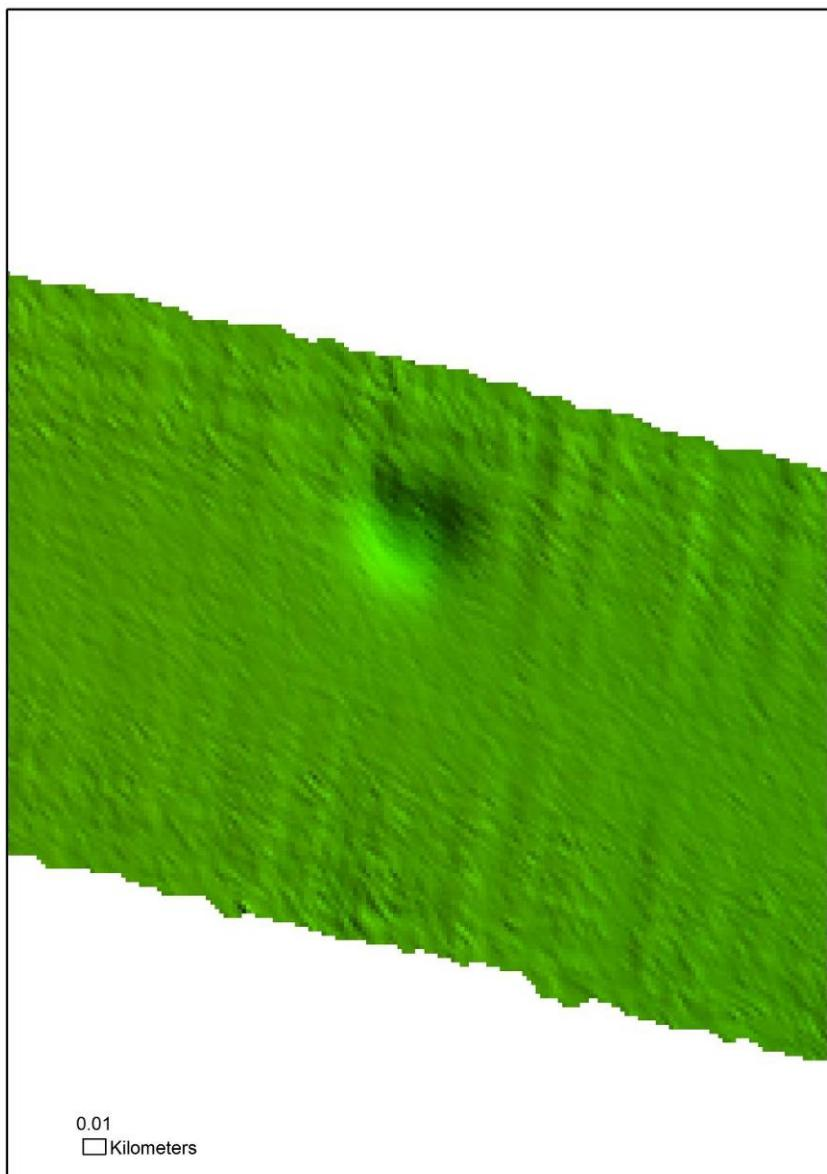
*Figure 13. Multibeam bathymetry showing a pockmark formed by shallow gas escape of which there were several in the area.*
