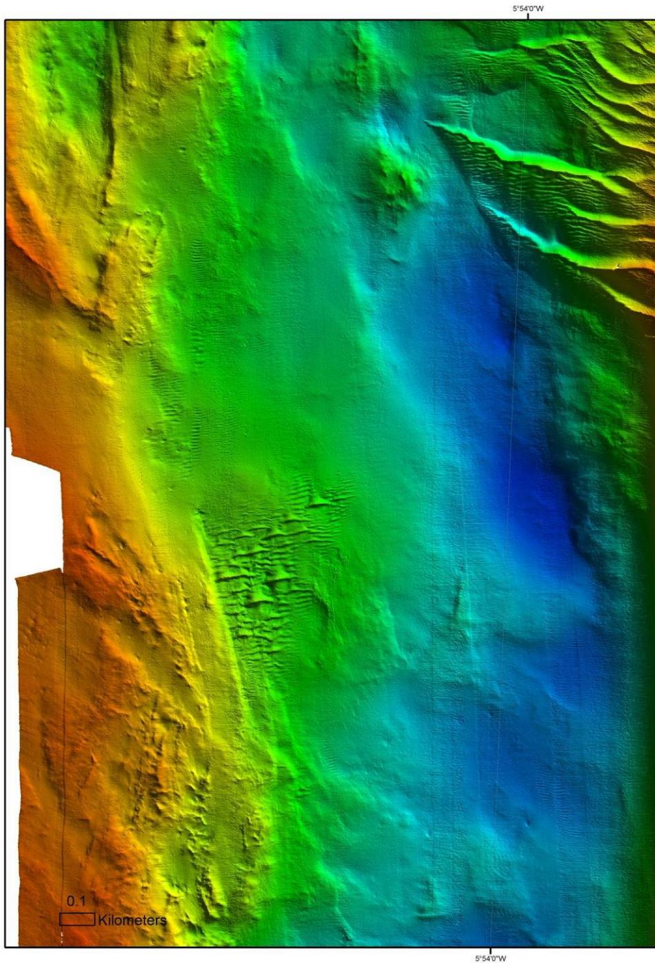
*Figure 39. Bathymetry map showing sediment waves of various sizes.*
