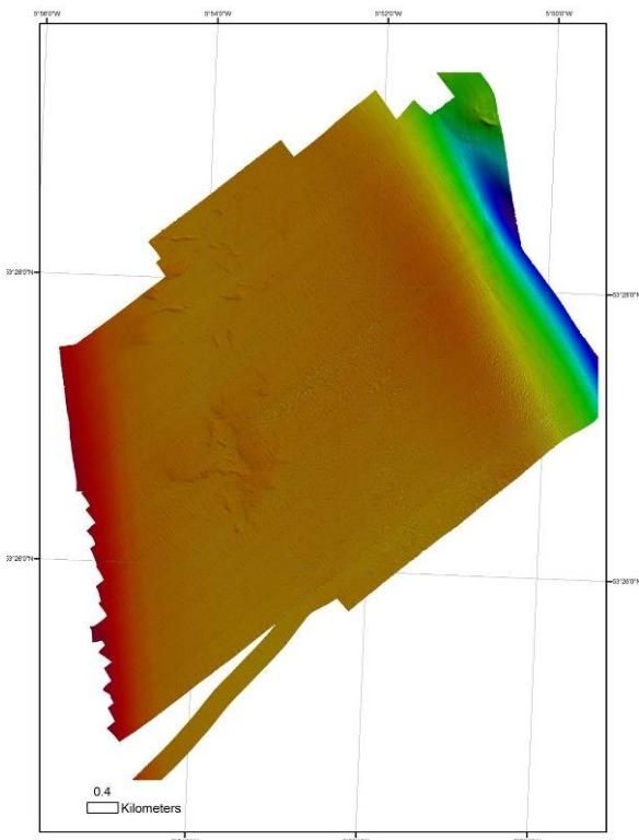
*Figure 28. Bathymetry showing gently sloping seabed and the Lambay deep to the east.*
