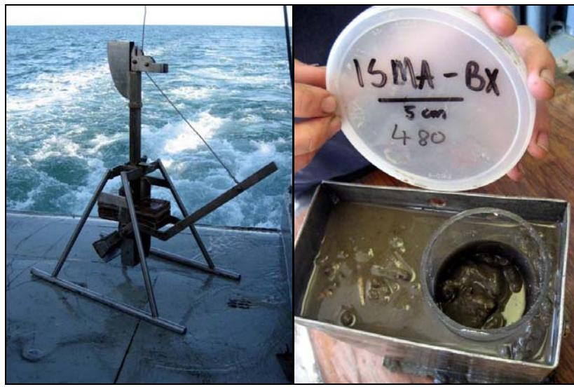
*Figure 8. The Reineck box-corer and retrieved sample showing the push-core inserted.*
