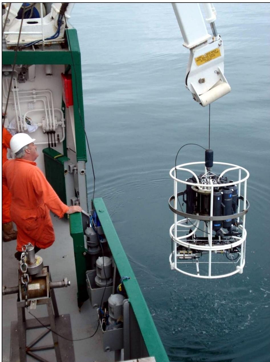
*Figure 5. Sea-Bird SBE 9plus CTD profiler being deployed*
