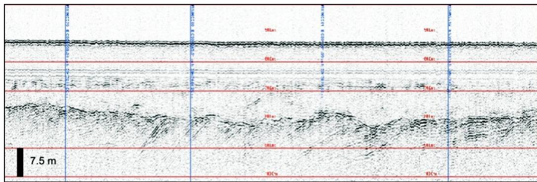
Figure 21. Seismic image showing bedrock 20 m below the surface. Dipping bedding is clearly discernable.
