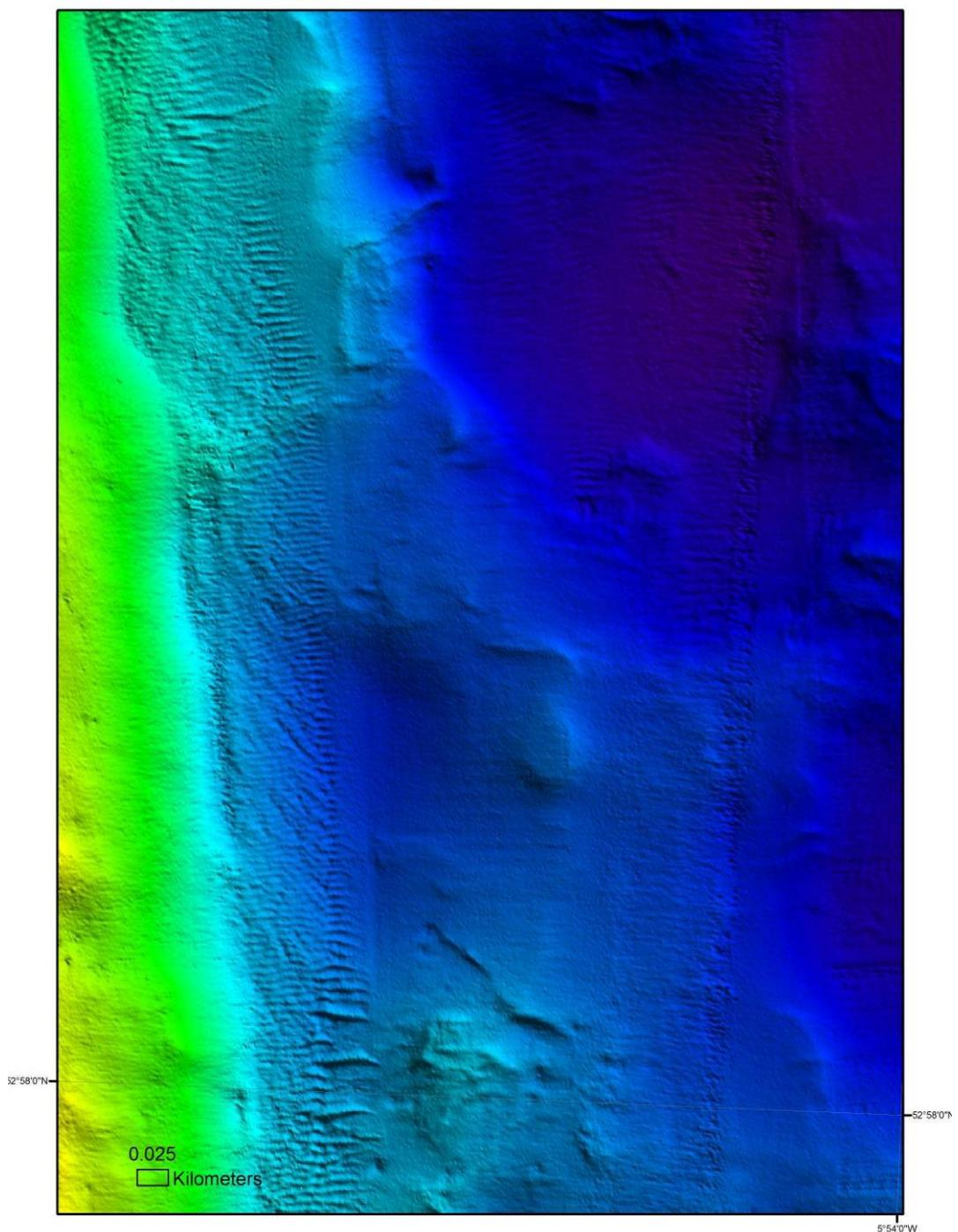
*Figure 41. Bathymetry map showing small scale sediment waves on the edge of the Codling Deep.*
