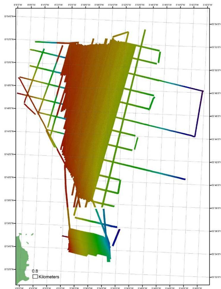
Figure 12. Multibeam bathymetric coverage in the Northern Mudbelt (northern and central coverage) and the Rockabill area (southern coverage). The image shows a smooth seabed, gentle sloping to the east.
