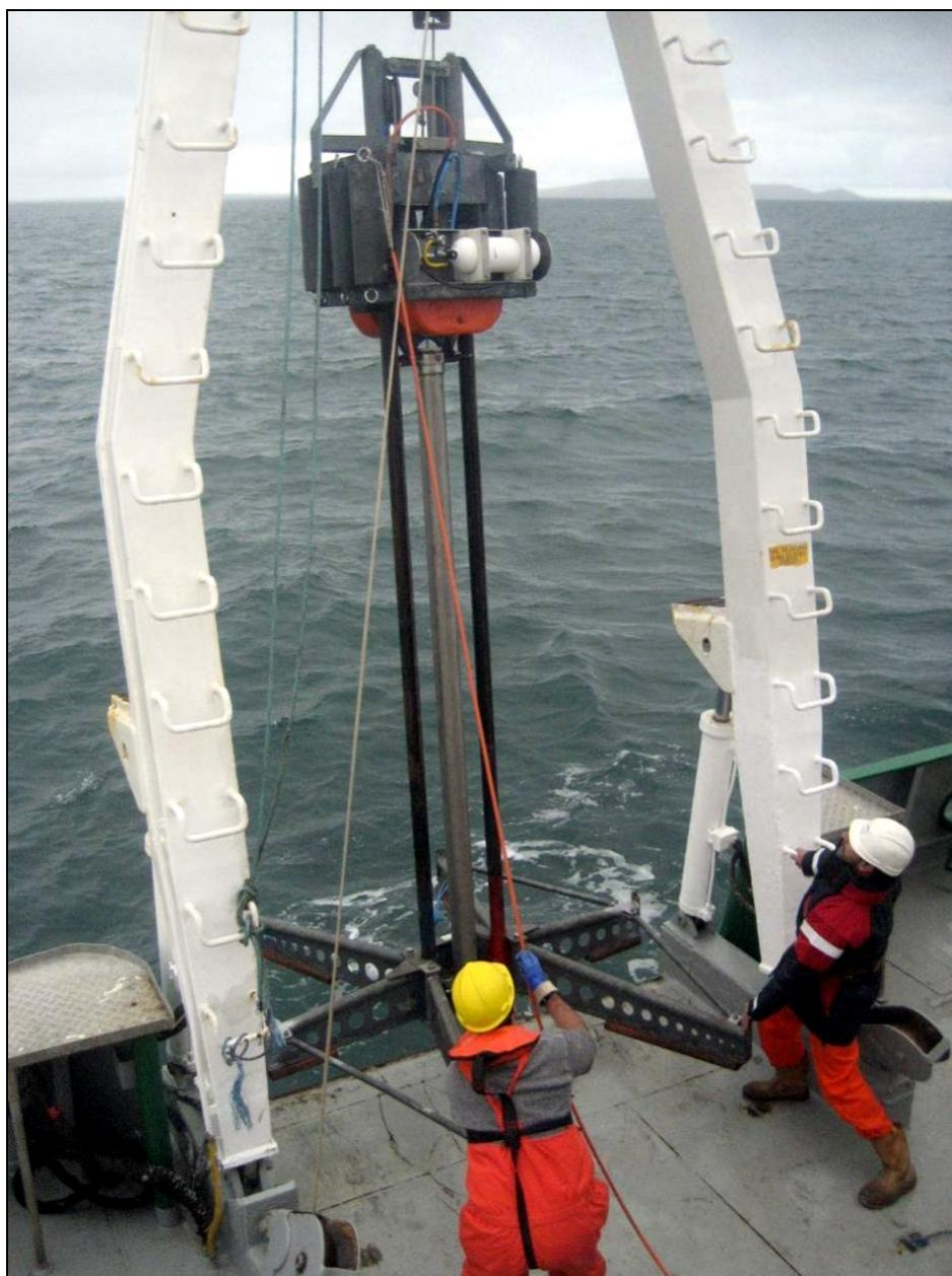
*Figure 10. The Geo-resources 6000 vibrocore being deployed*
