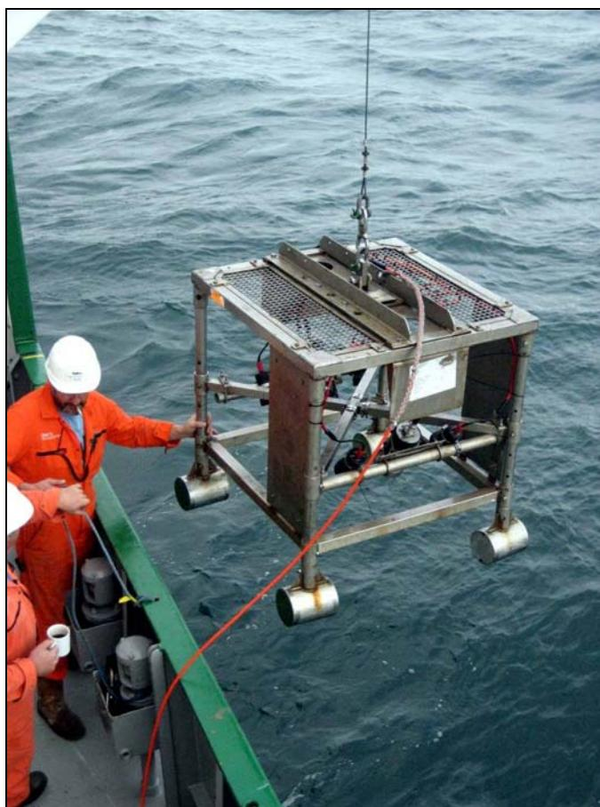
Figure 11. The digital stills camera, flash and LED lamps housed in the camera frame being deployed off the starboard winch during the survey
