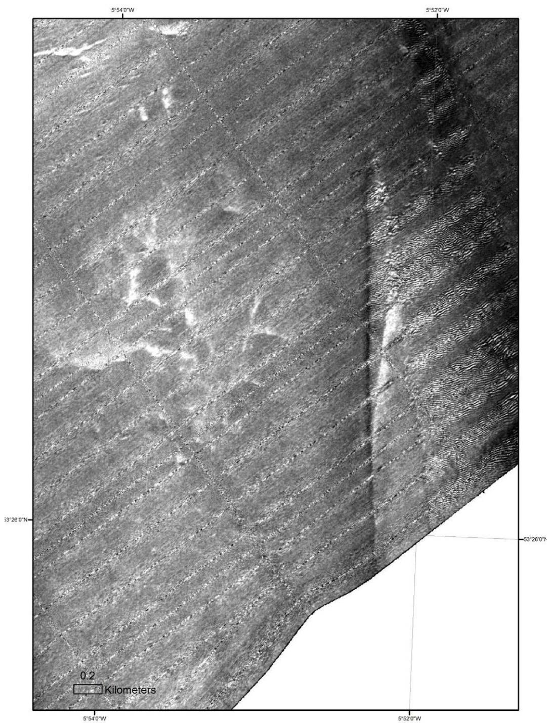
*Figure 30. Multibeam backscatter detail showing strong return (white) indicating lithified sediment outcropping and a linear north-south feature possibly a fault.*
