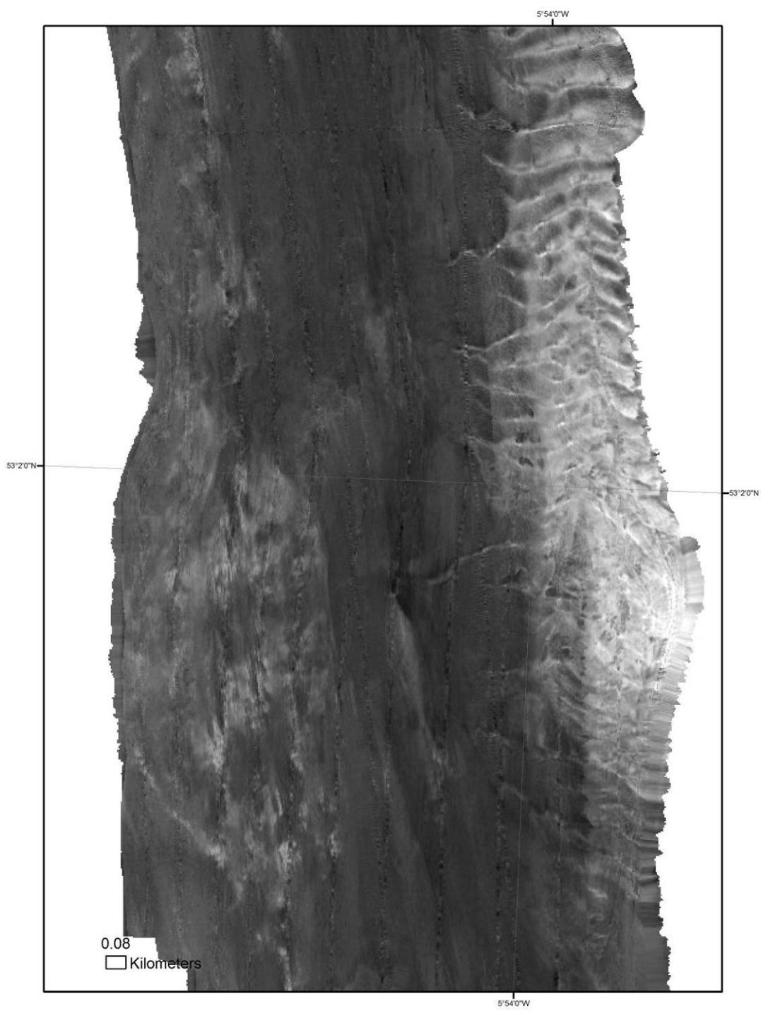
*Figure 40. Backscatter map showing sediment waves (right hand side) and mottled seabed covered with cobbles (left hand side).*
