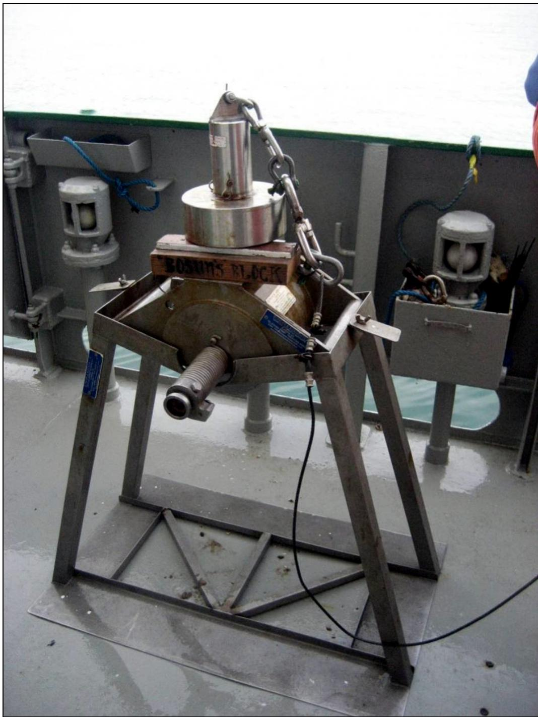
*Figure 7. Shipek sampler on stand*
