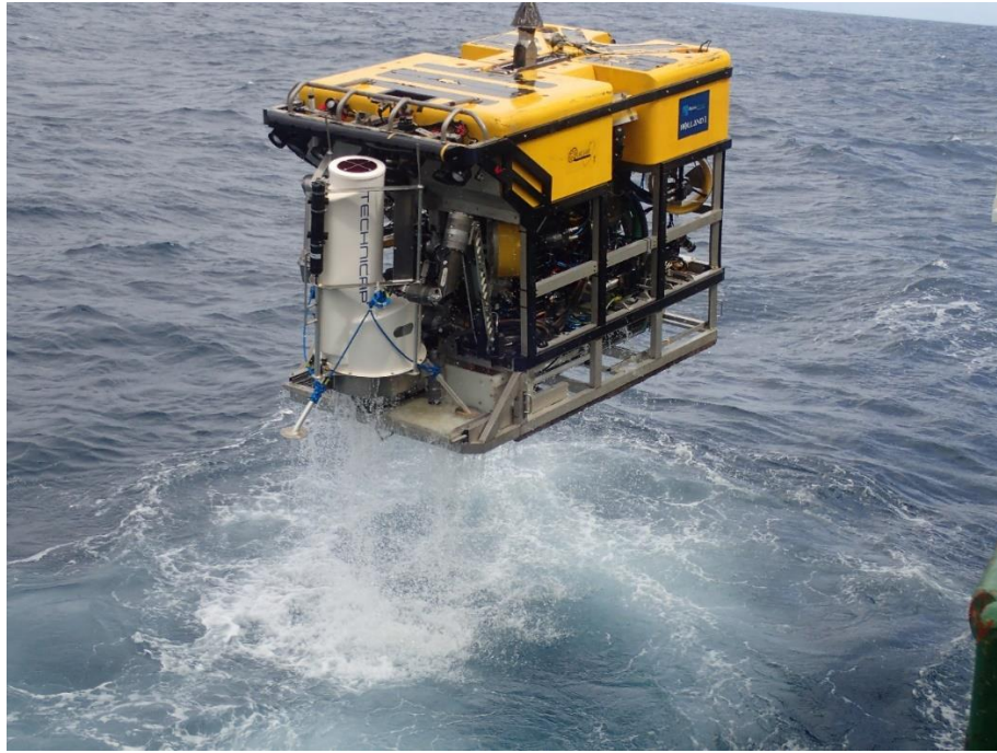
Holland 1 ROV retrieving one of the lander systems
