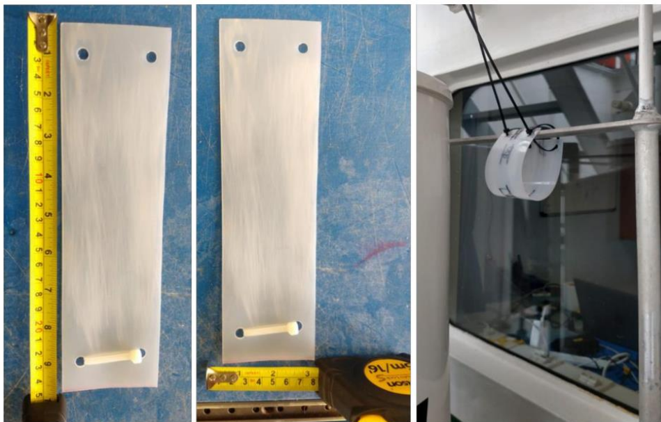
Nylon strips (measuring tape as scale - right). Nylon strip mounted on lander frame (left)
