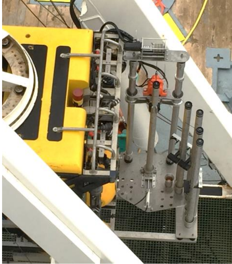
The vibrocorer mounted onto the front of the ROV
