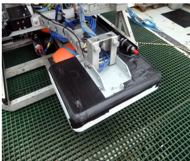
Kongsberg EM2040 mounted on the Holland 1 ROV
