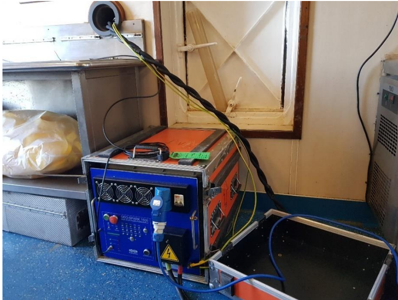
Figure 4: Sparker system bang box in the wet lab of the RV Celtic Voyager .
