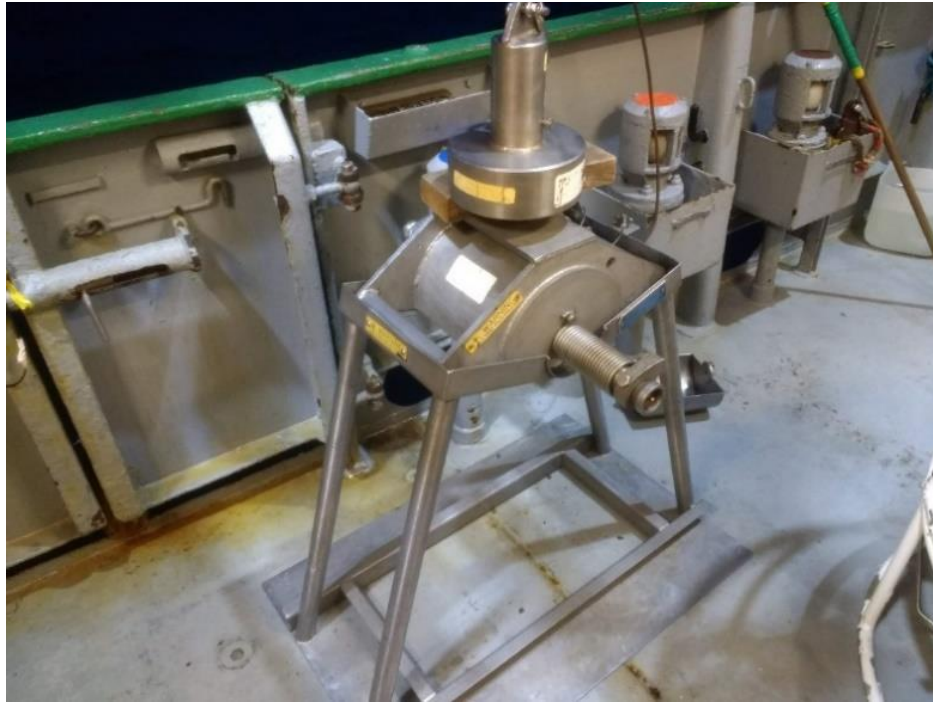
Figure 7: Shipek grab sampler, on its storage stand aboard the RV Celtic Voyager .
