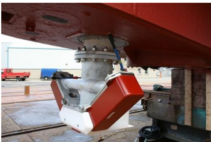
Figure 4: Kongsberg EM2040 Multibeam echosounder hull-mounted array. (Photo credit: Marine Institute, 2014.)
