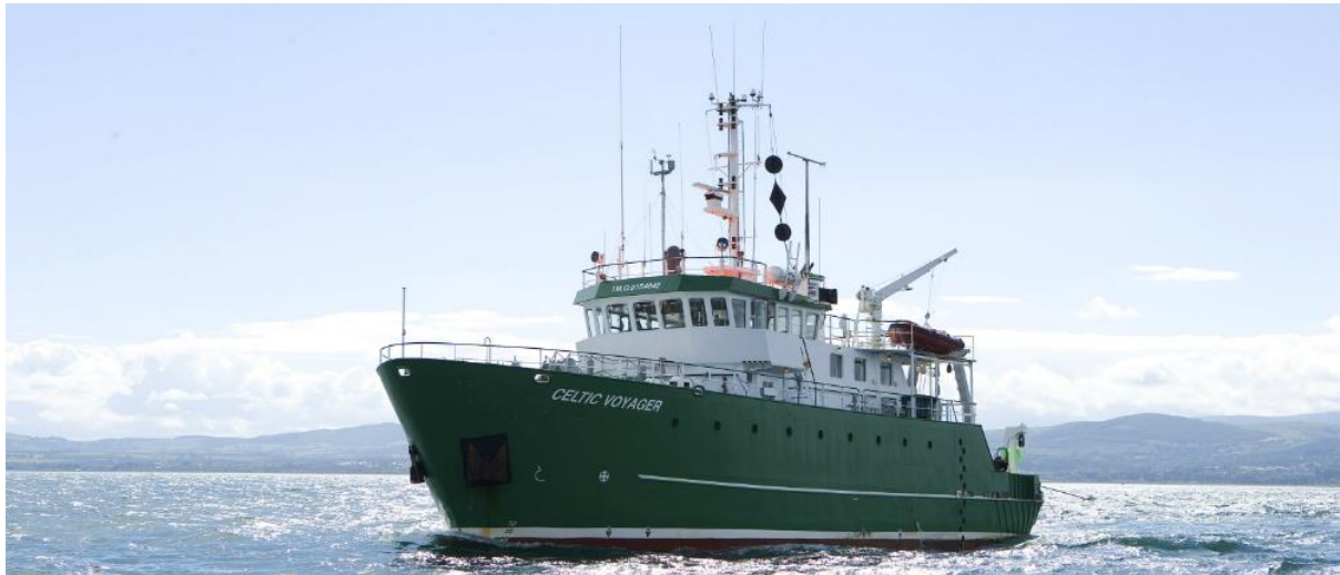
Figure 3: The RV Celtic Voyager, a 31.4 m, multi-purpose research vessel capable of oceanographic and environmental data collection. Photograph credit: Marine Institute.
