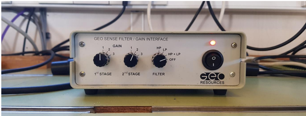
Figure 11: Geo Resources, filter/gain interface box with settings used during seismic data acquisition in area 3. Knobs from left: 1 st stage gain (set to 1); 2 nd stage gain (set to 2); and filter (set to HP + LP).
