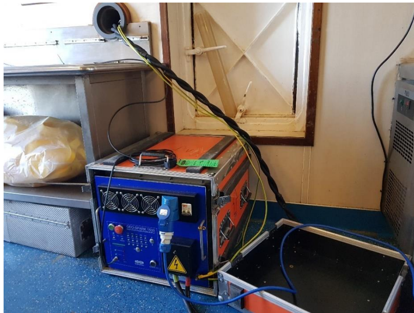
Figure 5: Sparker system bang box in the wet lab of the RV Celtic Voyager .
