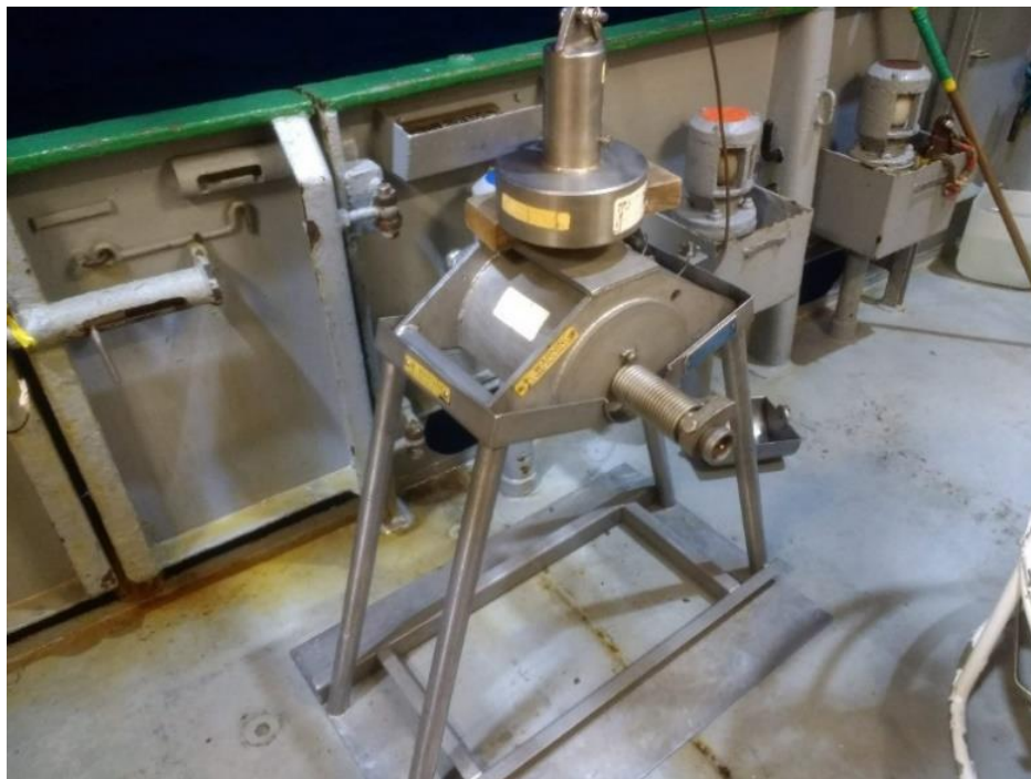
Figure 8: Shipek grab sampler, on its storage stand aboard the RV Celtic Voyager .
