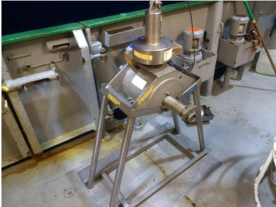
Figure 4: Shipek grab sampler, on its storage stand, used during the AggreWind research cruise (CV18034).
