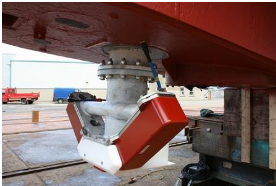
Figure 3: Kongsberg EM2040 Multibeam echosounder hull-mounted array. (Photo credit: Marine Institute, 2014.)
