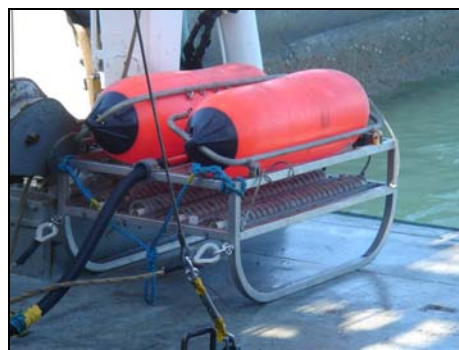
Figure 4. Geo-Spark 1500 power supply and towed Geo-Source 400 Sparker source
