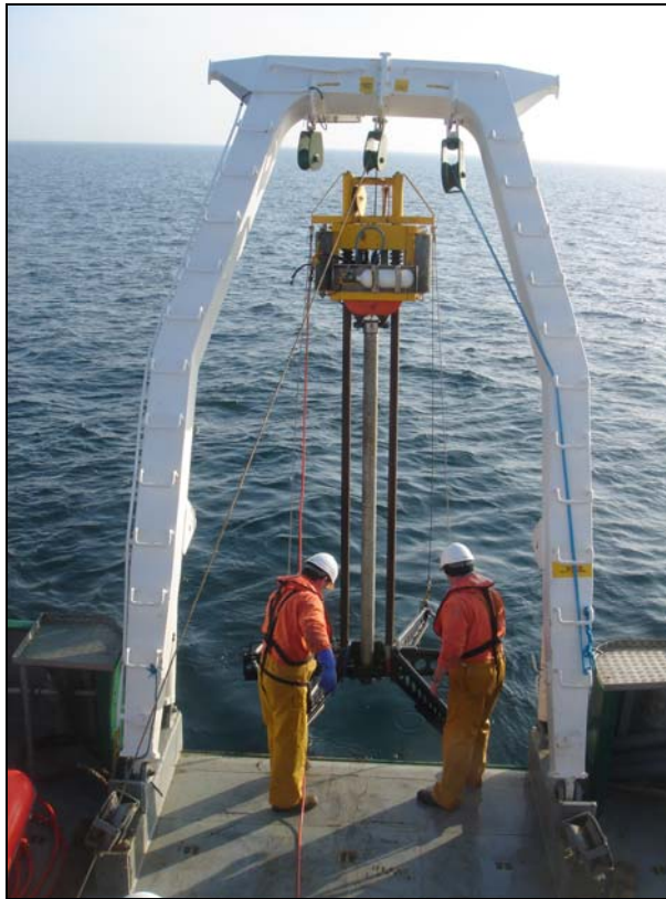
Figure 5. The Geo-resources 6000 vibrocore being deployed
