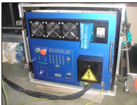
Figure 4. Geo-Spark 1500 power supply and towed Geo-Source 400 Sparker source
