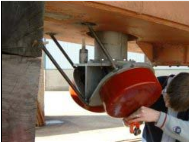
Figure 3. Hull mounted multibeam transducer on the RVCeltic Voyager (photo of the Marine Institute).
