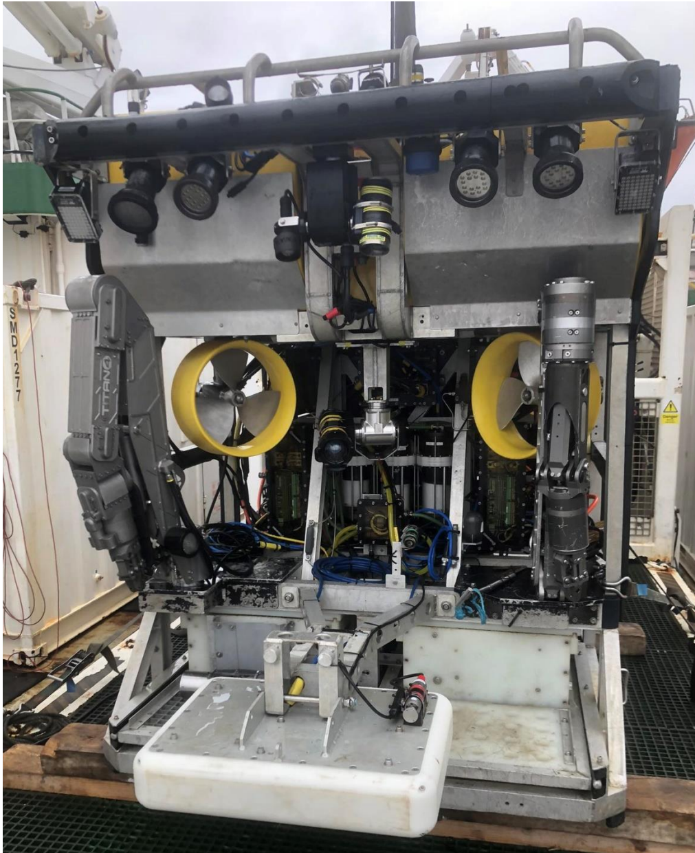
Figure 4. Holland 1 Remotely Operated Vehicle with the EM2020 multibeam echosounder head install on the front
