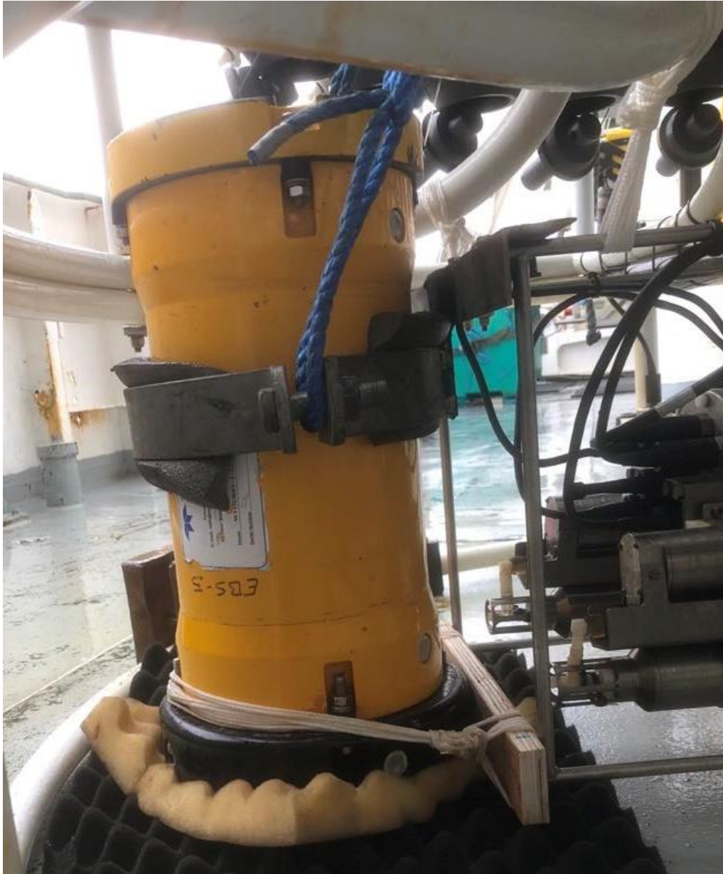
Figure 7. A Teledyne / RDI Workhorse 1 Sentinal 300 kHz ADCP bracketed to the CTD in a downward-facing L-APCD mode.
