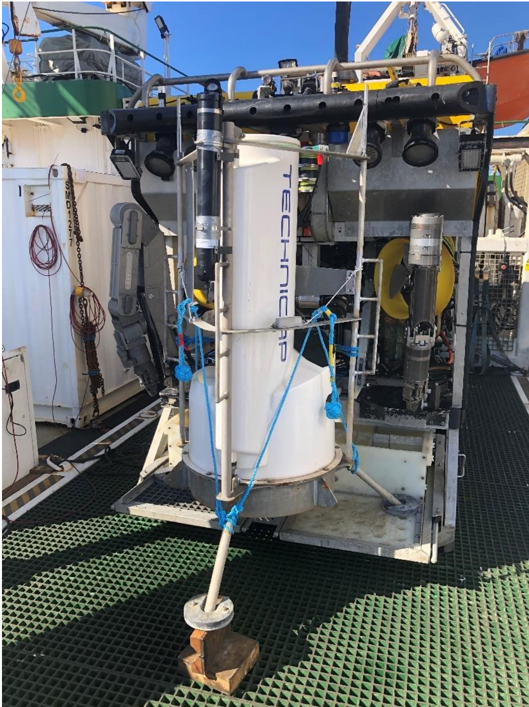
Figure 5. Little MonSta lander “Adele” ready for deployment on the front of the Holland 1 ROV
