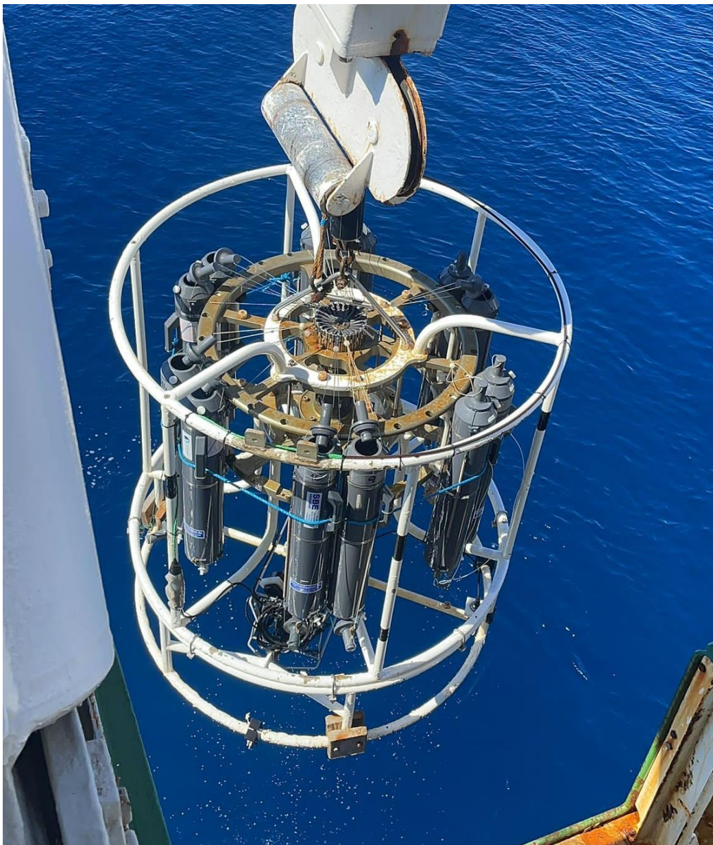
Figure 6. Sea Bird Electronics SBE 911 plus CTD
