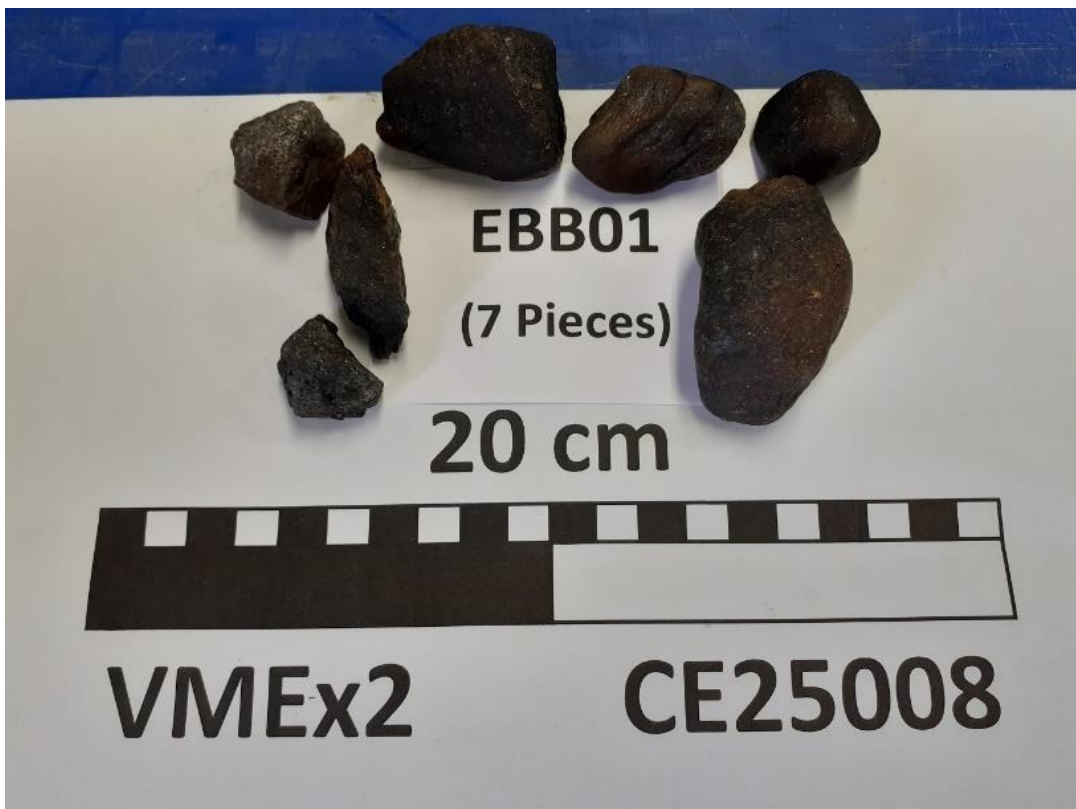
Figure 31. Station 56: Edoras Bank Middle rock dredge samples
