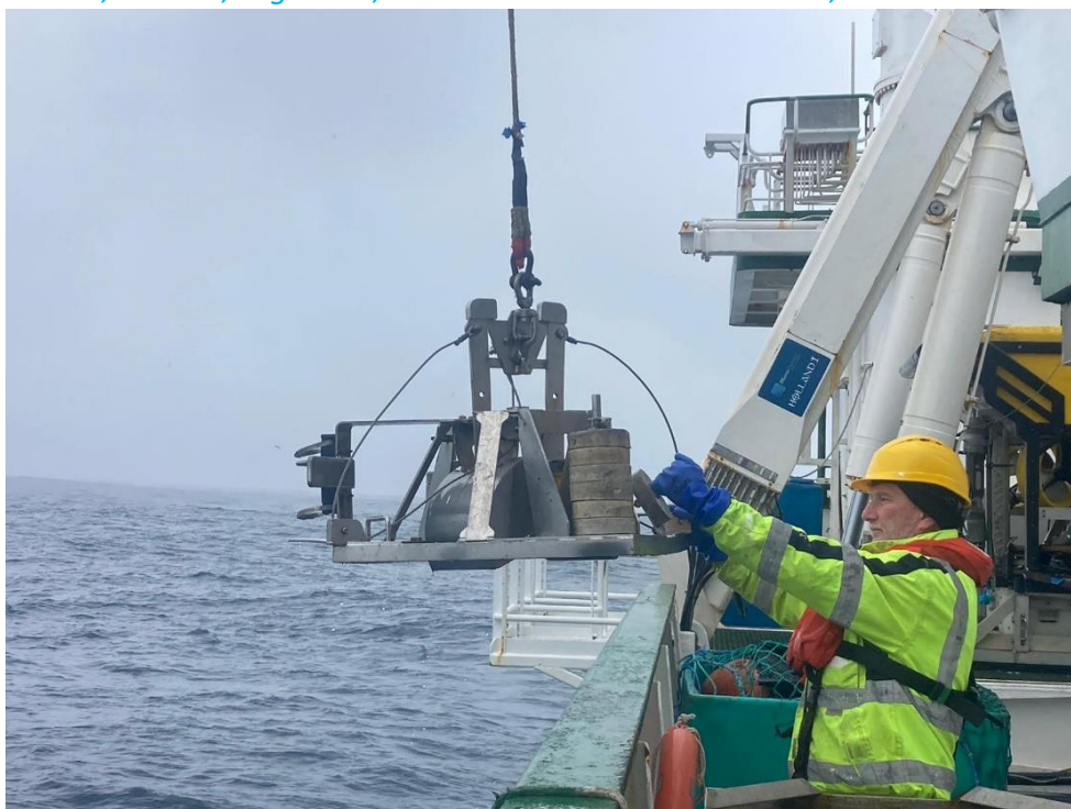
Figure 25. Day grab being deployed at Station 74.
