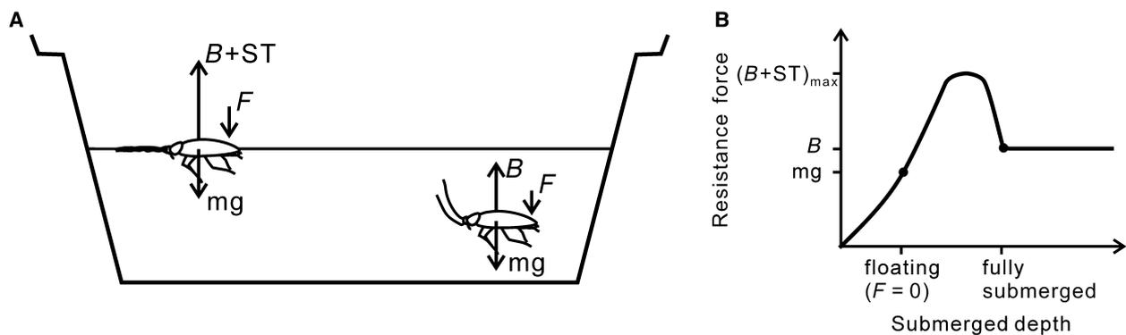
**FIG. 1.** Schematic diagrams showing: A, the forces exerted on floating and submerged carcasses; B, change in resistance force exerted by water on a carcass vs submerged depth. *Abbreviations:*  $B$ , buoyancy;  $ST$ , surface tension;  $F$ , external force;  $mg$ , weight.
