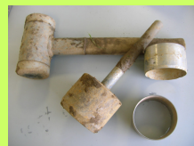
Figure 3: bulk density sampler
