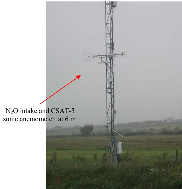
N<sub>2</sub>O intake and CSAT-3
