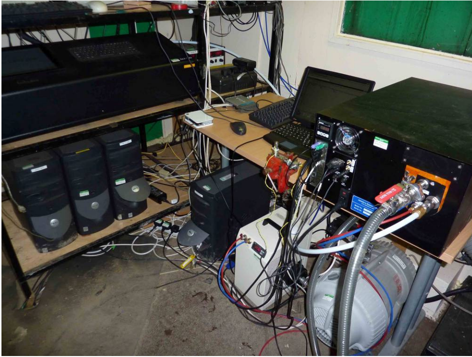
Figure 2: FR equipment including FMA (on the left), QCL (top right), cryogen cooler and pump are on the ground.
