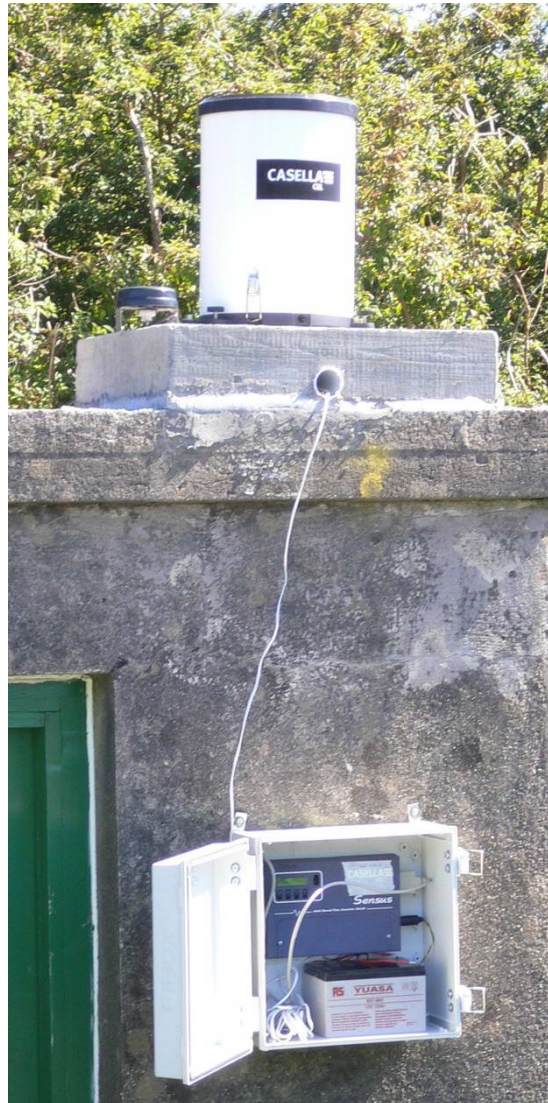
Figure 4.7 The raingauge and its data logger in Bweeng
