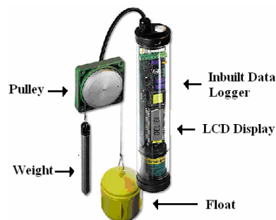
Figure 5.2 Thalimedes shaft encoder (Ott-Hydrometry, 2004)
