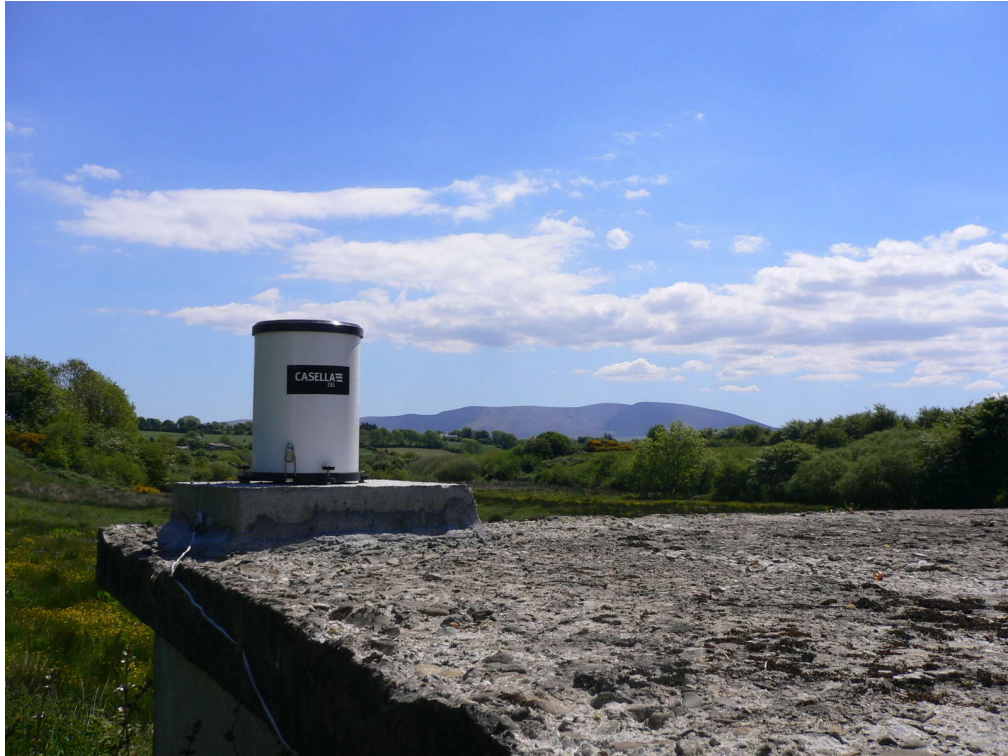
Figure 4.5 To avoid interception, the gauge is installed on the roof of a reservoir in Knocknagree
