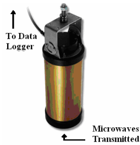
Figure 2-12 Kalesto Radar Sensor (Ott-Hydrometry, 2004)
