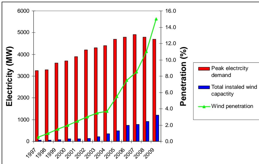
**Figure 5: Historical growth in Irish electricity demand, installed wind capacity and wind penetration (information from Eirgrid, (O'Leary, et al. 2007), (Howley, et al. 2008))**
