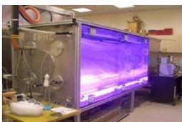
Figure 2. Atmospheric Simulation Chamber
