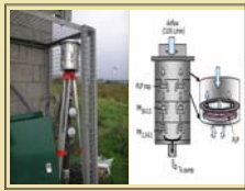
Fig 3. The three stage high volume cascade impactor, collecting PM 10-2.5 and PM 2.5 onto polyurethane foam.
