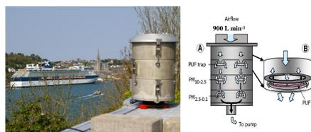
Figure 1. High Volume Cascade impactor
