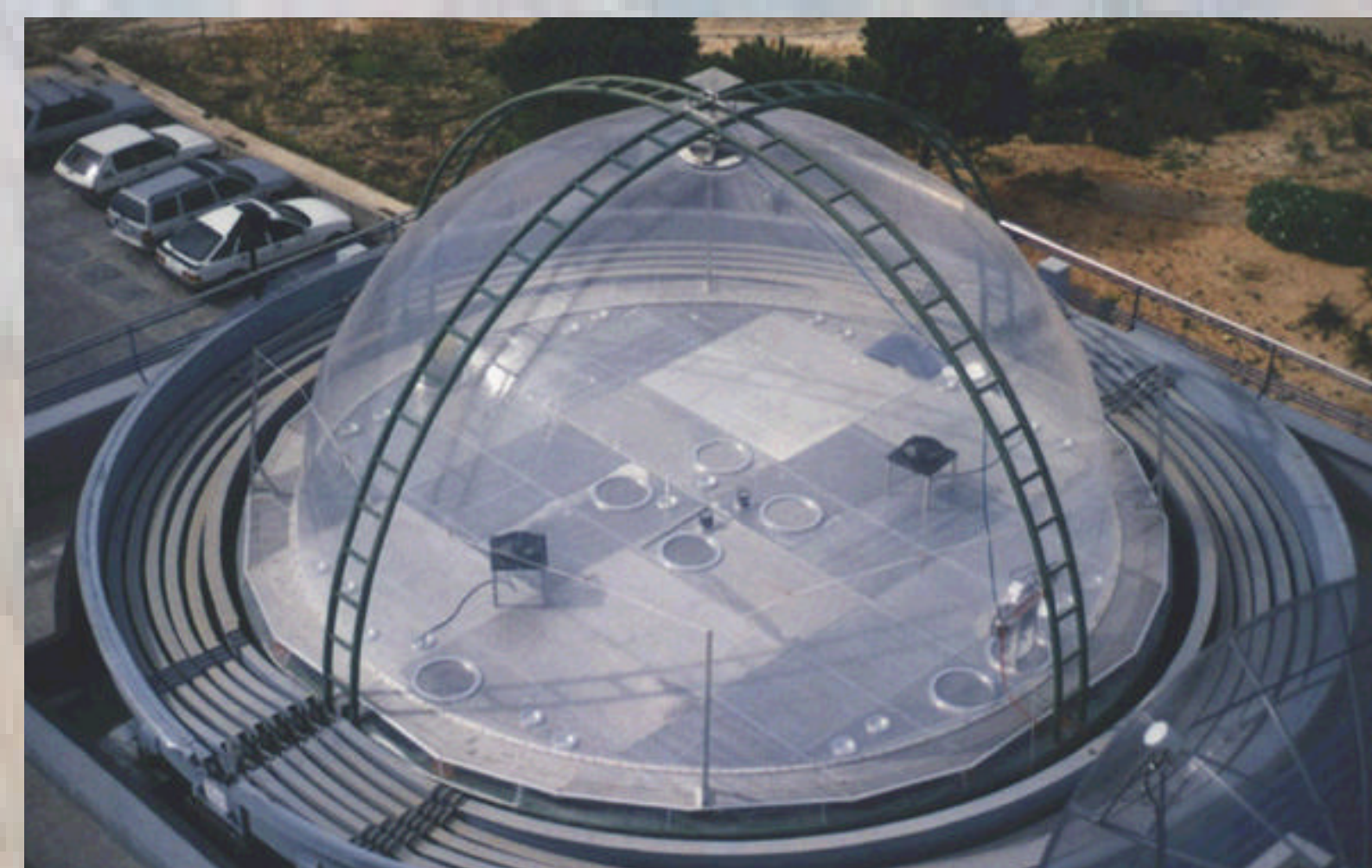
Figure 6: Chamber B of the EUPHORE facility Valencia, Spain
