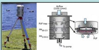
Fig 1. The three stage high volume cascade impactor, collecting PM<sub>10-2.5</sub> and PM<sub>2.5</sub> onto polyurethane foam.
