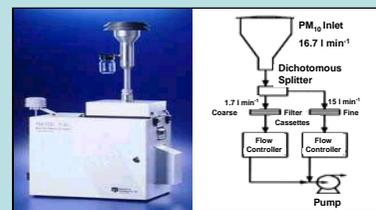
Fig 2. The Partisol sampler with the dichotomous splitter for the collection of PM<sub>10-2.5</sub> and PM<sub>2.5</sub> on PTFE filters.
