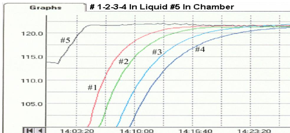
One can see that the autoclave chamber reaches 121°C approximately 3 minutes after the cycle has started. However, the lower portions of the liquid do not reach 121°C until the cycle has run for almost 20 minutes. It is important to keep in mind that the liquid was not at 121°C for a majority of the cycle duration.
