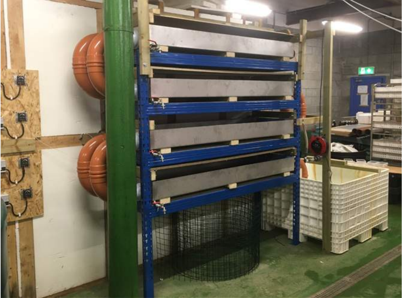
A view of the intermediate duckweed cultivation system at BEES, UCC. This system will allow us to better understand the challenges of up-scaling duckweed growth, and will be operated at a capacity of up to 600 litres.
