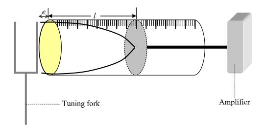
Beginning with the highest frequency tuning fork and a very short column of air, adjust the piston until the sound from the vibrating air column is loudest; this is the first resonance point. Measure the length l of the air column at resonance. Proceed to use the set of tuning forks to complete the data table as in the previous method (it is difficult to distinguish resonance for frequencies below 340 Hz).
