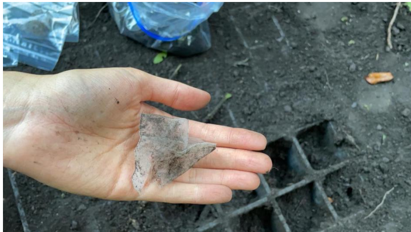
Figure 5. Image of a Tesco Finest Green Jasmin Pyramid Tea 15S 30G teabag, made of the bioplastic PLA, being recovered completely intact after 12 months in soil.
