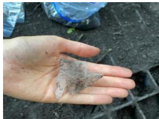
Figure 2: Image of a ‘Tesco Finest Green Jasmin Pyramid Tea 15S 30G’ teabag, made of the bioplastic polylactic acid (PLA), being recovered completely intact after 12 months in Irish garden soil.
