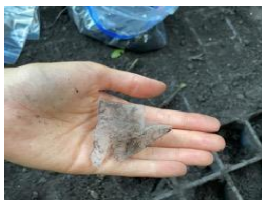
Figure 2: Image of a ‘Tesco Finest Green Jasmin Pyramid Tea 15S 30G’ teabag, made of the bioplastic polylactic acid (PLA), being recovered completely intact after 12 months in Irish garden soil.
