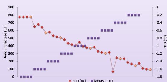
Figure 6: Graph of freezing point depression (FPD) of 4.8% lactose with increasing amounts of Colief lactase enzyme
