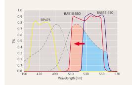
The new IBA cube is optimized to maximize both GFP excitation and detection of GFP emission through the use of a new dichroic mirror with minimal crossover.
