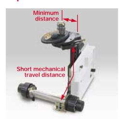
Short mechanical circuit structure and high rigidity nosepiece design avoids pitching and yawing when the nosepiece is manipulated during operations such as DIC prism insertion or adjustment of an objective's correction collar.
