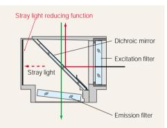
When the fluorescence excitation light is reflected by the dichroic mirror, some light may pass through the mirror and reflect as stray light in the cube assembly. This stray light may reflect out of the cube and into the imaging path, resulting in decreased contrast due to autofluorescence. Low reflection materials are incorporated into the design of all new Olympus fluorescence filter cubes. Such a design absorbs over 99% of all stray light, resulting in high contrast fluorescence images.
