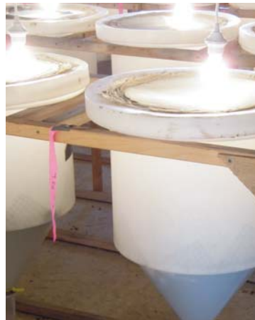
Beresele funnel invertebrate extractors. The litter samples are placed inside and over three days the invertebrates migrate away from the light and heat of the 100 watt bulb falling into the collection bag at the bottom.
