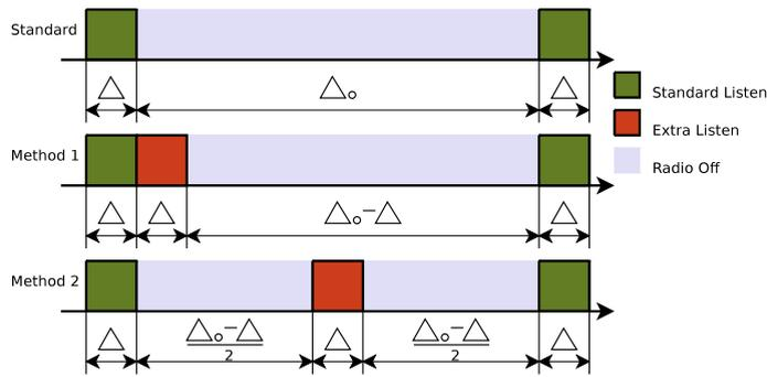
Fig. 5. Adaptive duty cycle.
