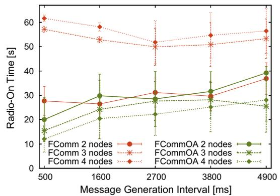
(b) Radio-on time for FrameComm and FrameCommOA for 2, 3, and 4 leaf nodes
