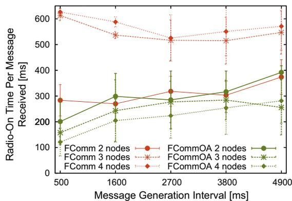
(c) Radio-on time per message received for FrameComm and FrameCommOA for 2, 3, and 4 leaf nodes
