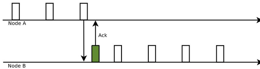
Fig. 3. Gaining the channel after carrier sense.
