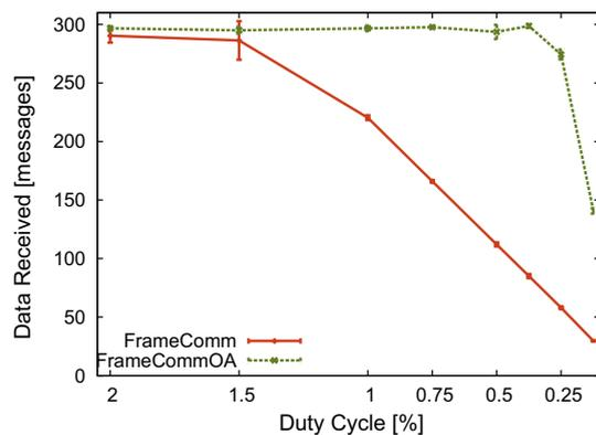
Fig. 11. The effects of reducing the duty cycle on data reception.
