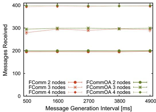
(a) Data delivered by FrameComm and FrameCommOA for 2, 3, and 4 leaf nodes
