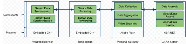
Figure 2. Software Architecture
