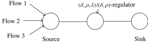
Fig. 3. The simulation topology with only one  $(\sigma, \rho, \lambda)/(\sigma, \rho)$ -regulated end host.
