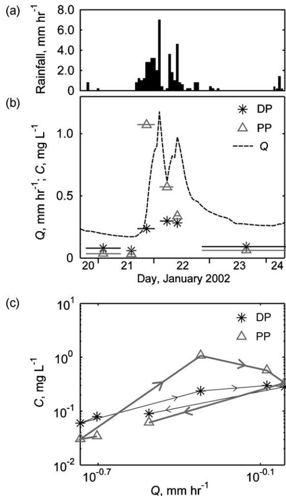
Fig. 8. An individual storm event, showing (a) rainfall, and (b) discharge and concentrations of dissolved phosphorus (DP) and particulate phosphorus (PP) in the stream water. The bars associated with the concentrations represent the span of time over which the composite sampling took place, and (c) *C* – *Q* plot for DP and PP, with PP exhibiting the greatest degree of hysteresis. Arrows represent the direction of the sequence through time.
