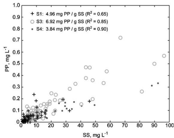
Fig. 4. Particulate phosphorus (PP) concentrations as a function of the suspended solid (SS) concentrations measured in the streams. The slope of the regression line is a measure of the phosphorus enrichment of the suspended solids.
