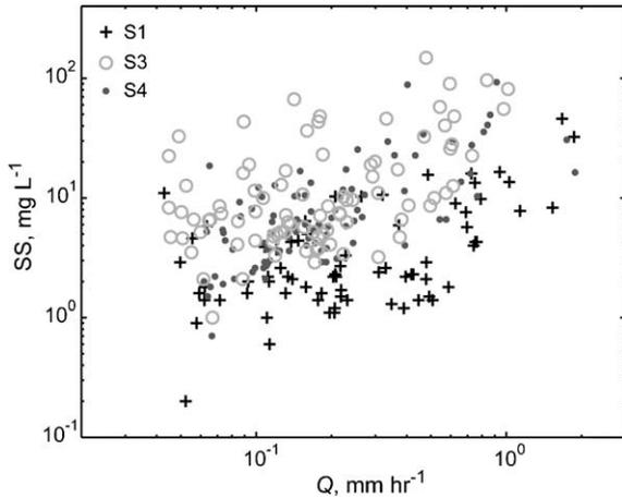
Fig. 5. Suspended solids (SS) as a function of discharge ( $Q$ ), showing stratification of the data according to site.
