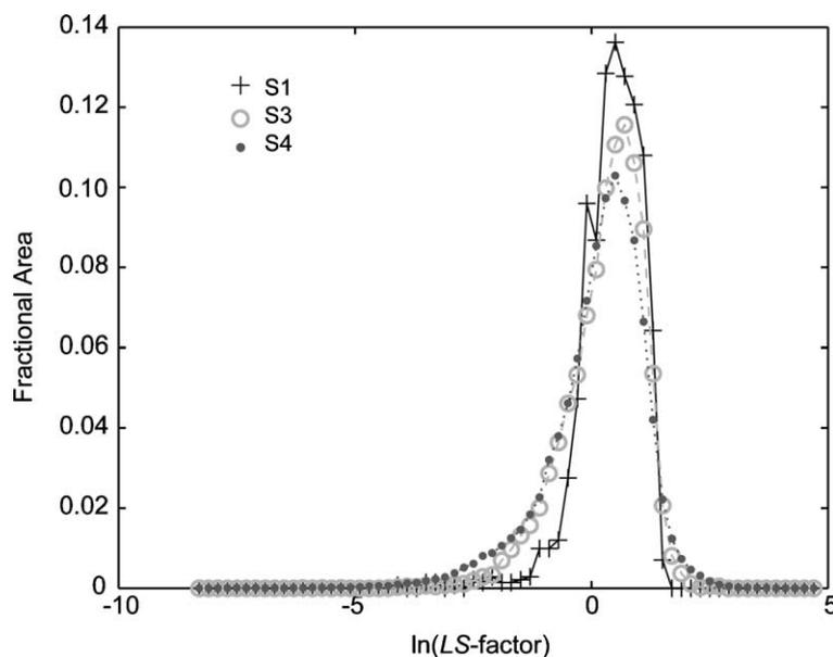
Fig. 7. PDF of the natural logarithm of the length–slope ( $LS$ ) factor, which is used as a descriptor of erosion potential for the sub-catchments.
