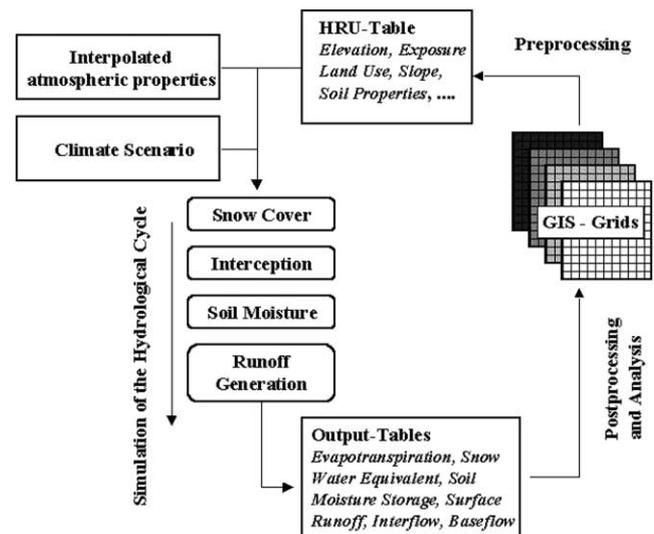
Fig. 4. Scheme of the hydrological catchment model PREVAH (Gurtz et al., 1999).
