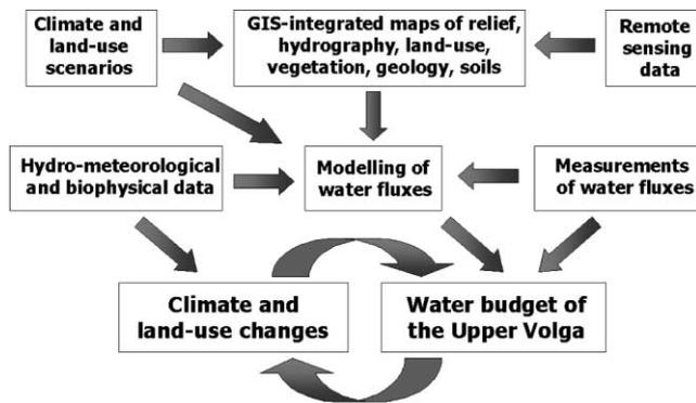
Fig. 1. A diagram of interrelation between different research activities to evaluate the response of the water budget of the boreal forest region at the Upper Volga area to climatic and land-use changes.
