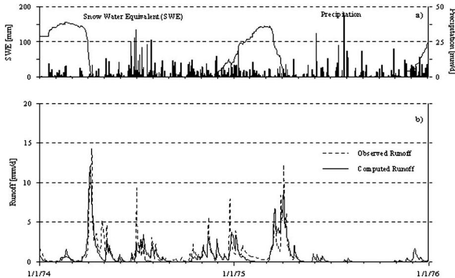
Fig. 11. Comparison of modelled (PREVAH) and measured (Usadievsky catchment) total runoff for period from 1974 to 1976.
