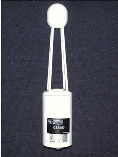
**Figure 2.9:** LI-7500 Open path CO<sub>2</sub>/H<sub>2</sub>O gas analyser
