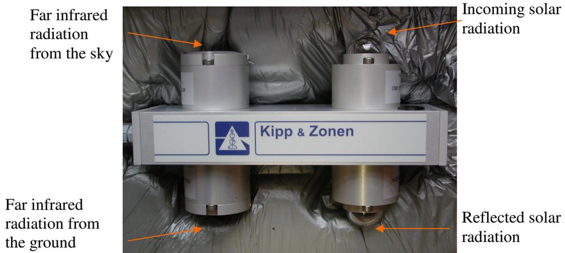
**Figure 2.8:** Net radiometer and its main components
