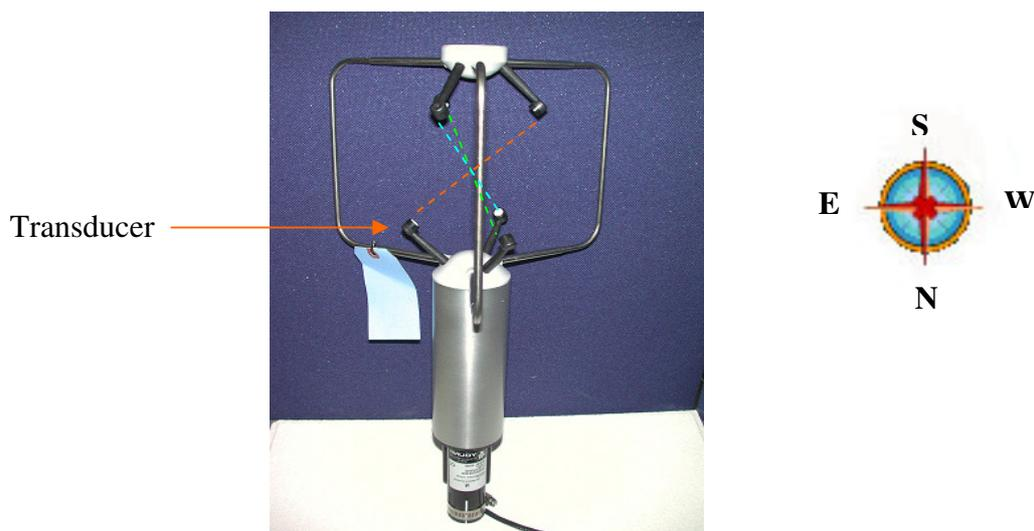
**Figure 2.7:** the sonic anemometer with the three paths shown in red (E -W), blue (SW-NE), green (NW-SE), as for a typical orientation of the device
