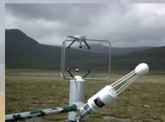
Figure 4. 3D Sonic anemometer and open-path CO<sub>2</sub>/H<sub>2</sub>O gas analyser
