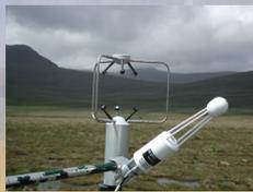
Figure 4. 3D Sonic anemometer and open-path CO<sub>2</sub>/H<sub>2</sub>O gas analyser
