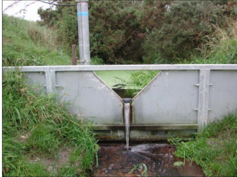
**Figure 2.14** The 90° V notch weir to measure stream flow at site 1.
