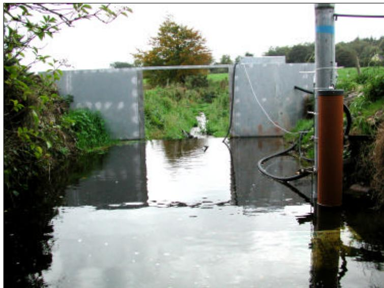
**Figure 2.15** The rectangular weir to measure stream flow at site 3.
