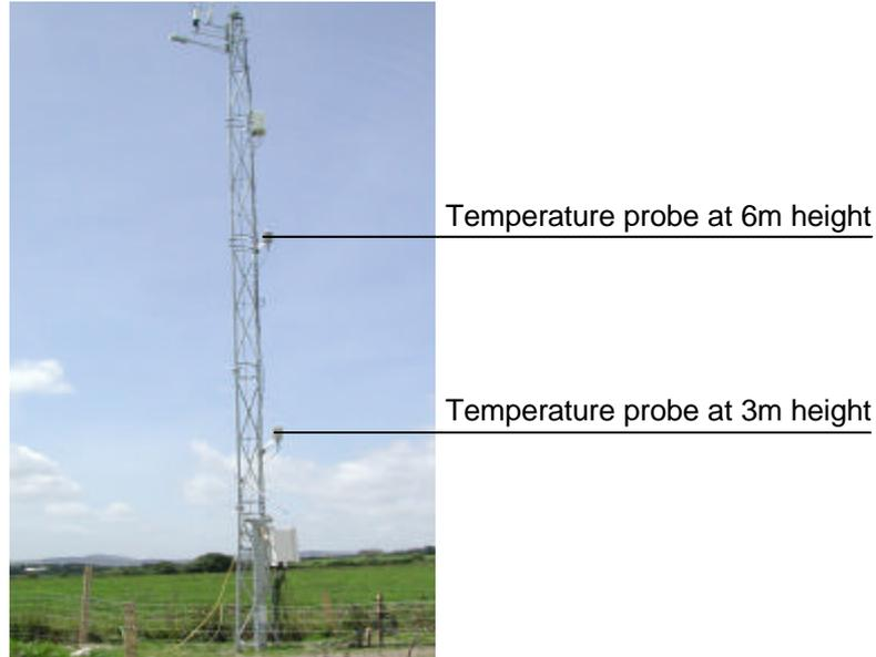
**Figure 2.6** The temperature probes in the 10 m meteorological tower.
