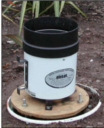
**Figure 2.9** The tipping bucket rain gauge.
